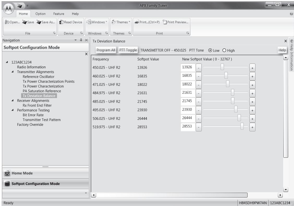
Figure 6-19. Transmit Deviation Balance Alignment Screen (UHF2)
