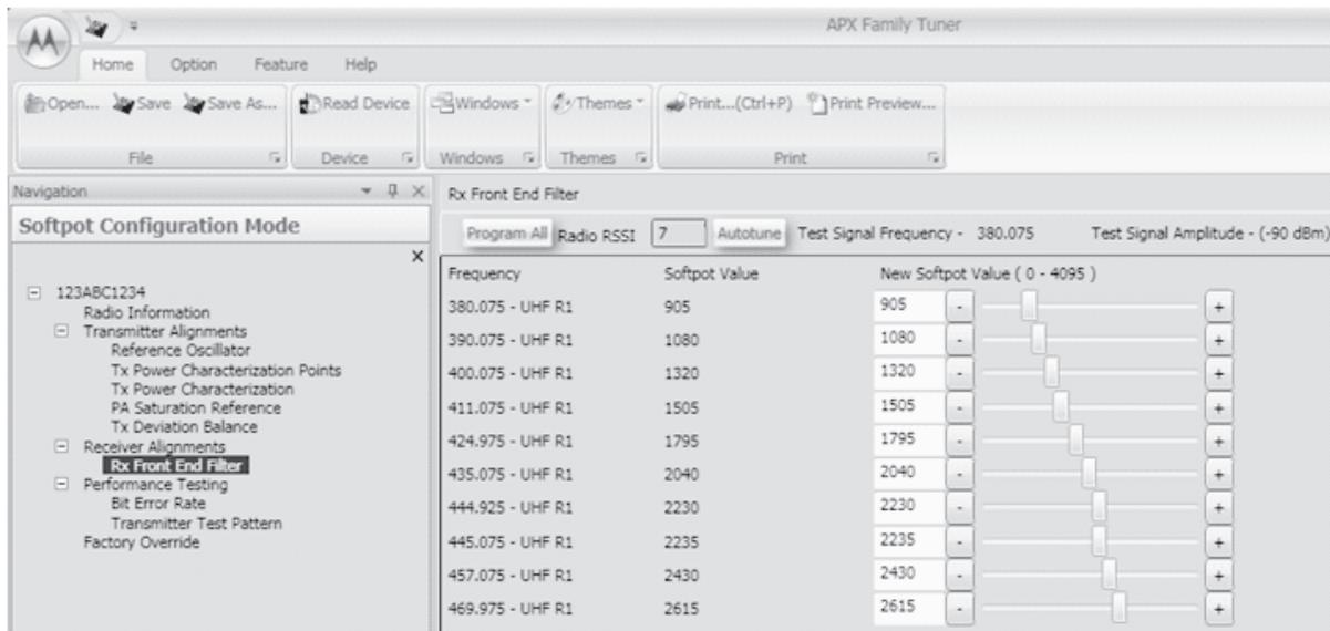
Figure 6-30. Front End Filter Alignment Screen (UHF1)
