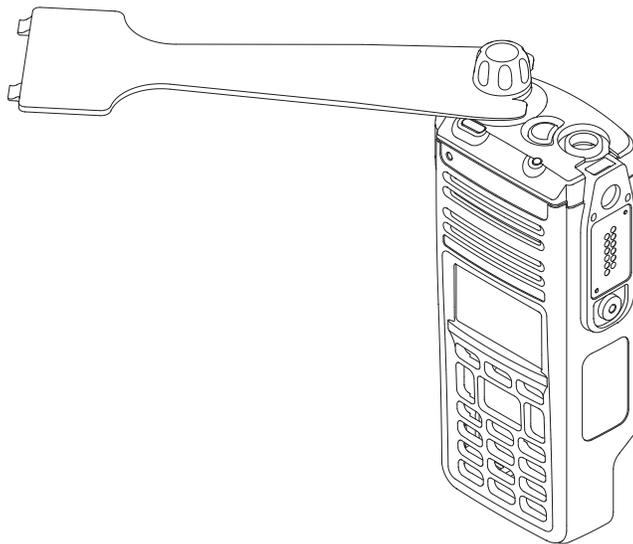
*Figure 7-25. Servicing the Multi Function Knob*
