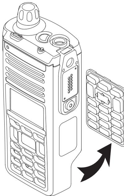
*Figure 7-21. Remove the Keypad*
