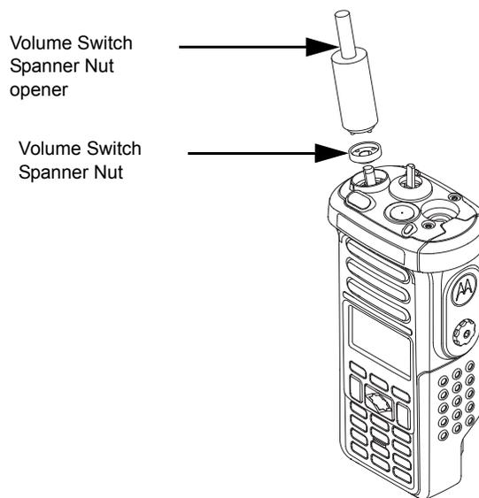
Figure 8-46. Tighten the Volume Switch Spanner Nut
