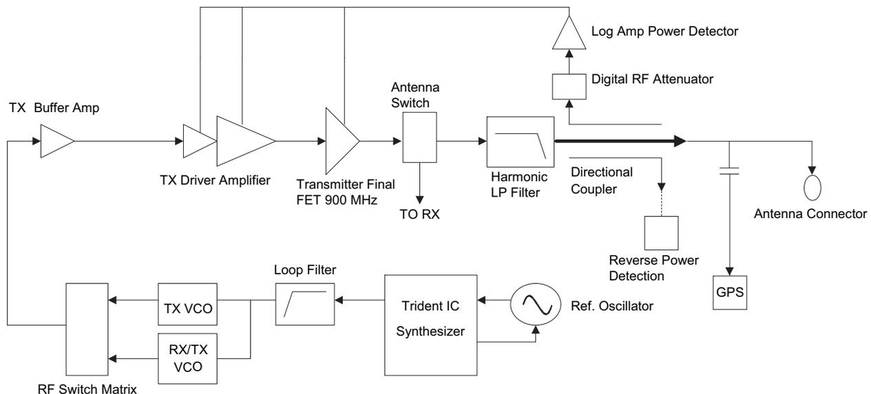
Figure 3-4. Transmitter (900 MHz) Block Diagram
