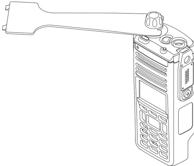
*Figure 7-24. Servicing the Multi Function Knob*
