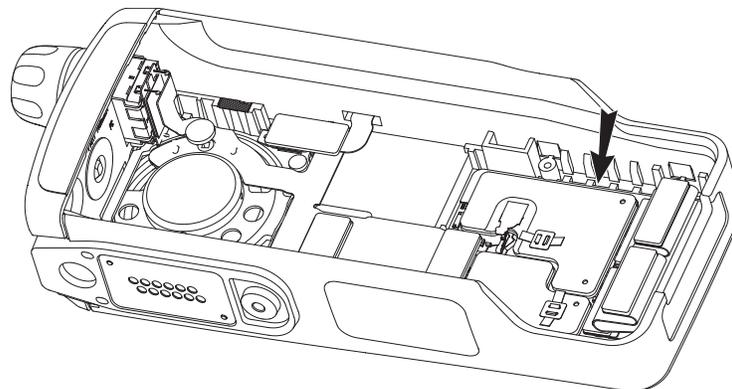
*Figure 8-19. Remove the Keypad Board*
