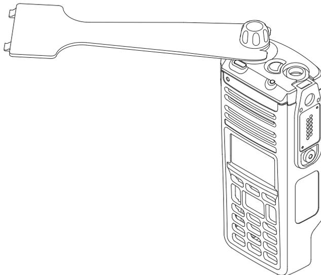
Figure 8-25. Servicing the Multi Function Knob
