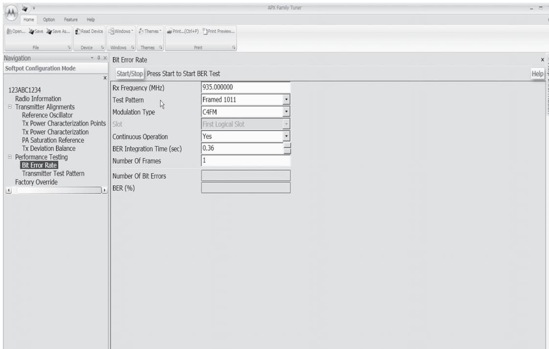
Figure 6-36. Bit Error Rate Screen (900 MHz)
