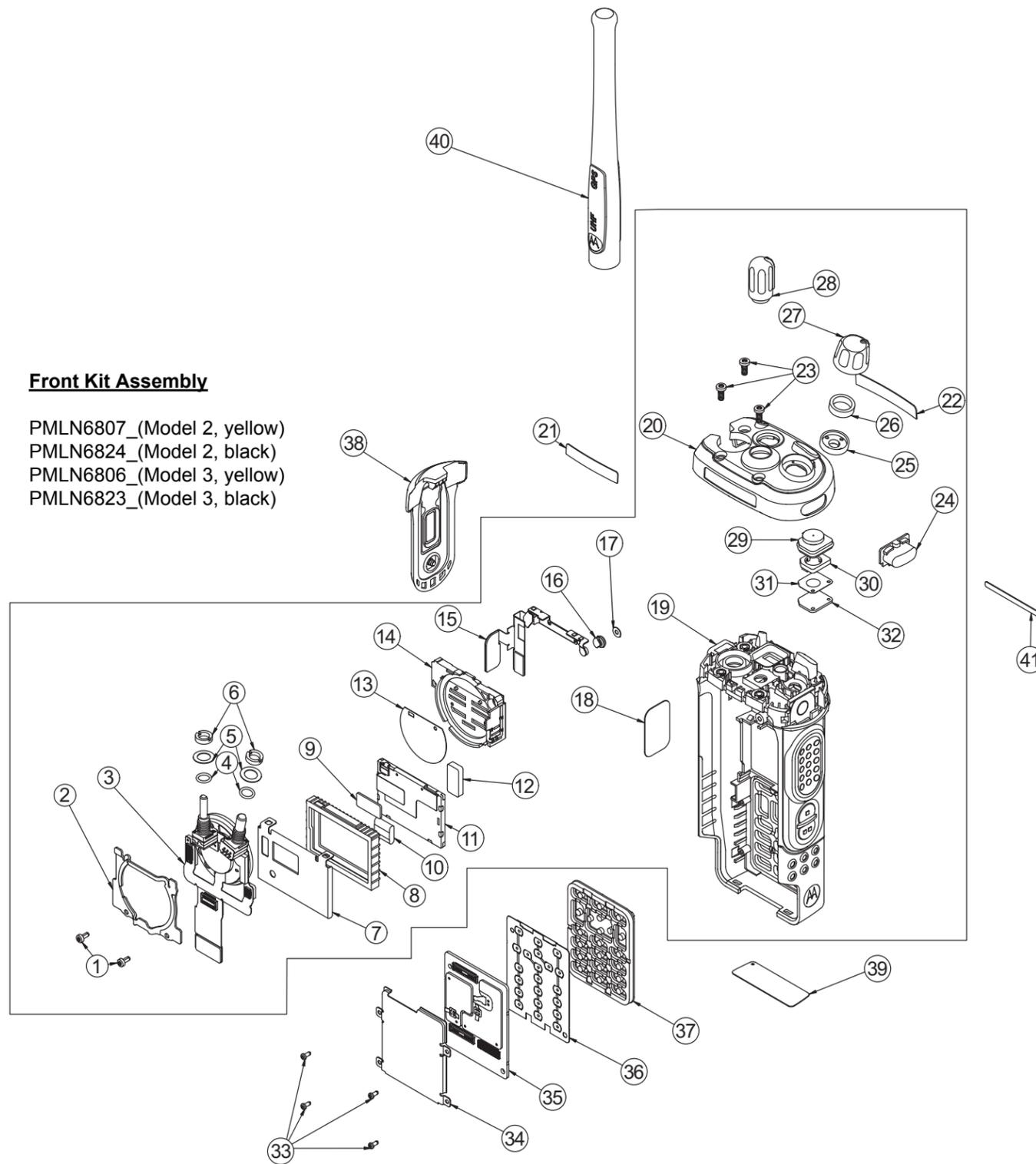
Figure 10-1. APX 2000/ APX 4000 (Two Knobs) Front Kit Exploded View
