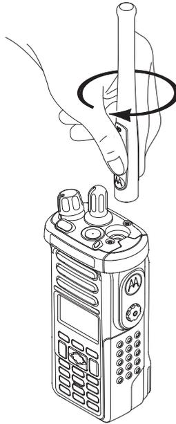
Figure 8-50. Attaching the Antenna
