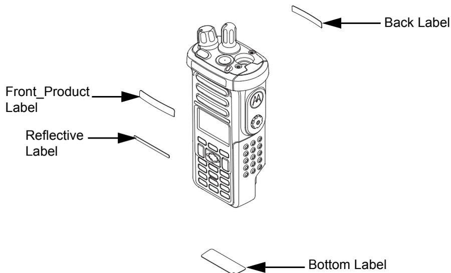
Figure 8-27. Serviceable Components – Main Housing
