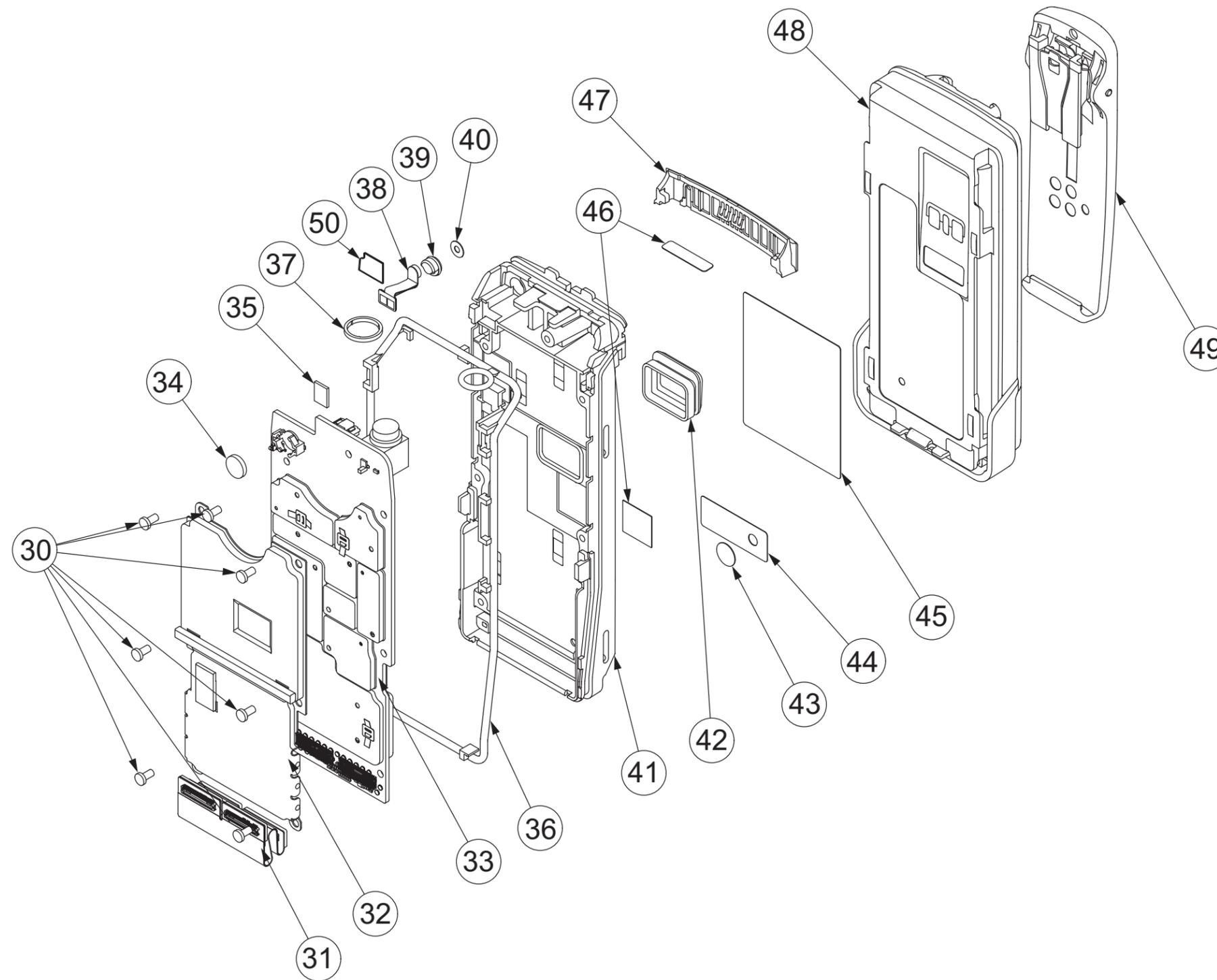
Figure 10-2. APX 2000/ APX 4000/ APX 4000Li Back Kit Exploded View
