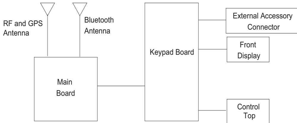
Figure 3-1. APX 2000/APX 4000/APX 4000Li Overall Block Diagram
