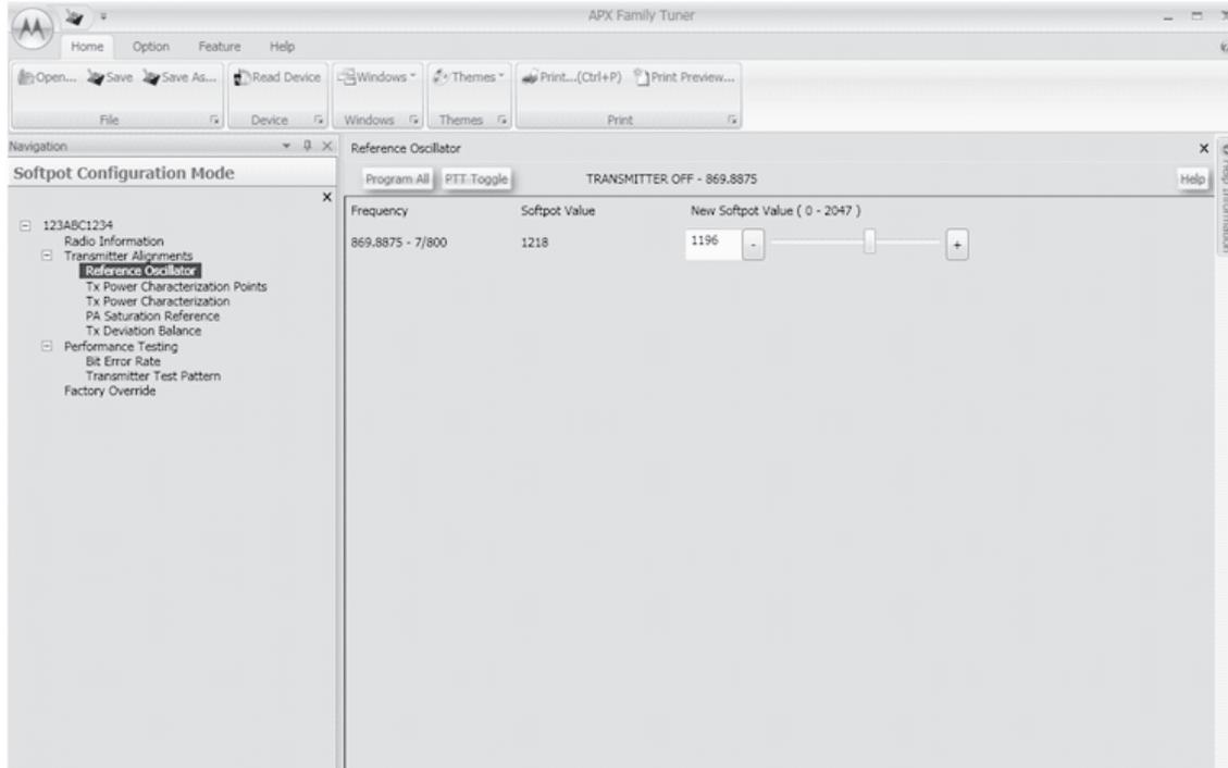
Figure 6-8. Reference Oscillator Alignment Screen (700/800 MHz)
