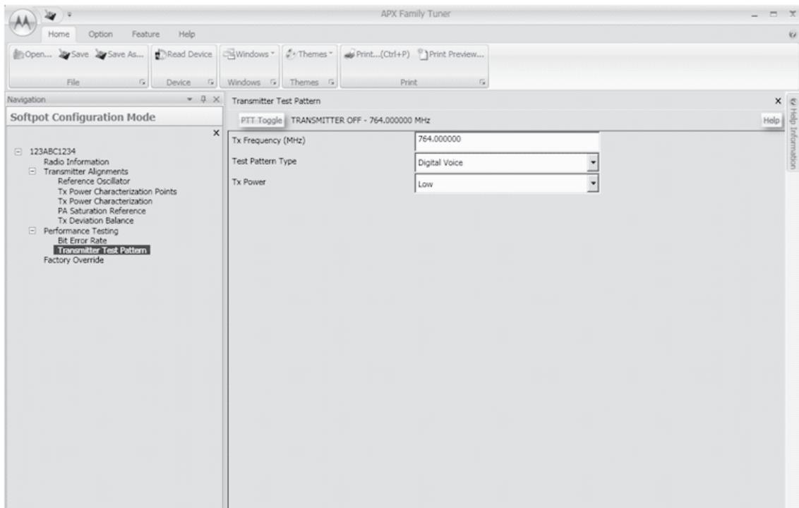
Figure 6-40. Transmitter Test Pattern Screen (700/800 MHz)
