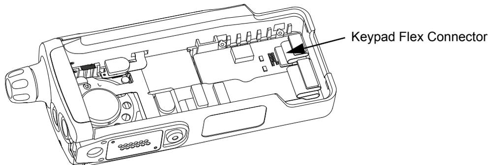
Figure 7-27. Rest the Front Kit Flex and plug in the Keypad Flex Connector
