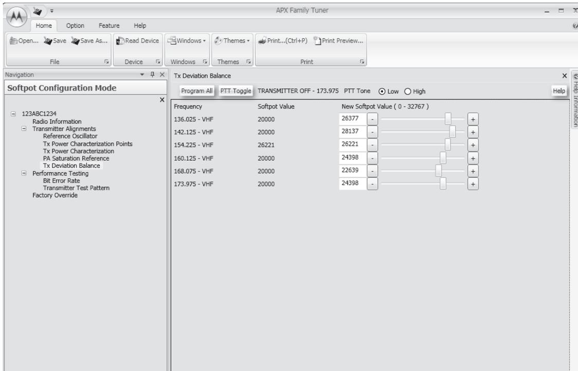
Figure 6-17. Transmit Deviation Balance Alignment Screen (VHF)
