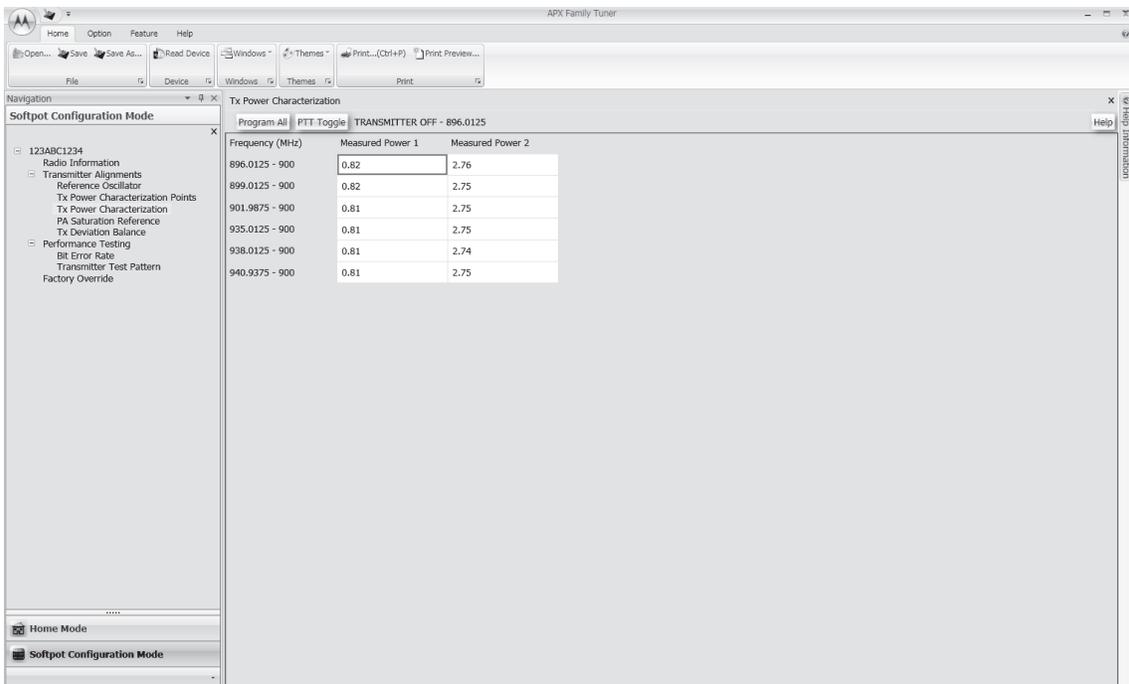
Figure 6-19. Transmit Power Characterization Alignment Screen (900 MHz)
