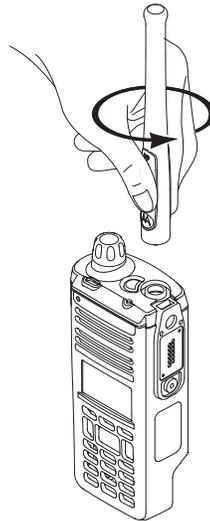
Figure 7-4. Removing the Antenna
