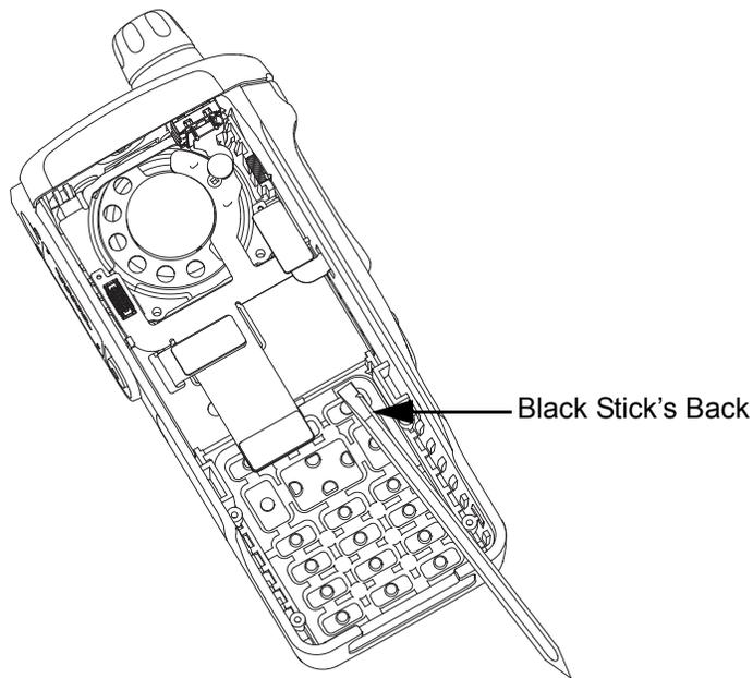
*Figure 7-30. Assemble the Keypad*
