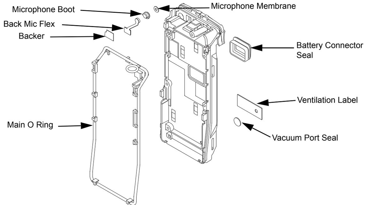
Figure 8-26. Serviceable Components – Chassis Assembly
