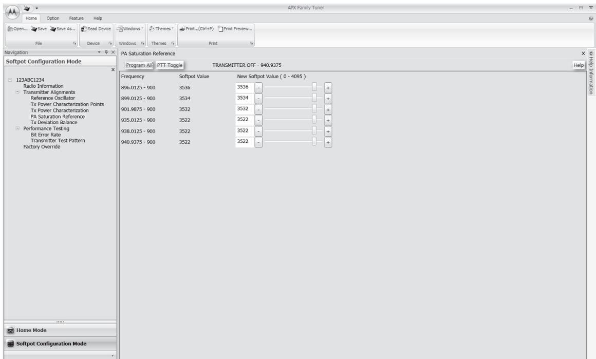
Figure 6-24. PA Saturation Referencing Alignment Screen (900 MHz)
