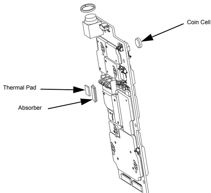
Figure 7-21. Serviceable Components – Main Board Assembly
