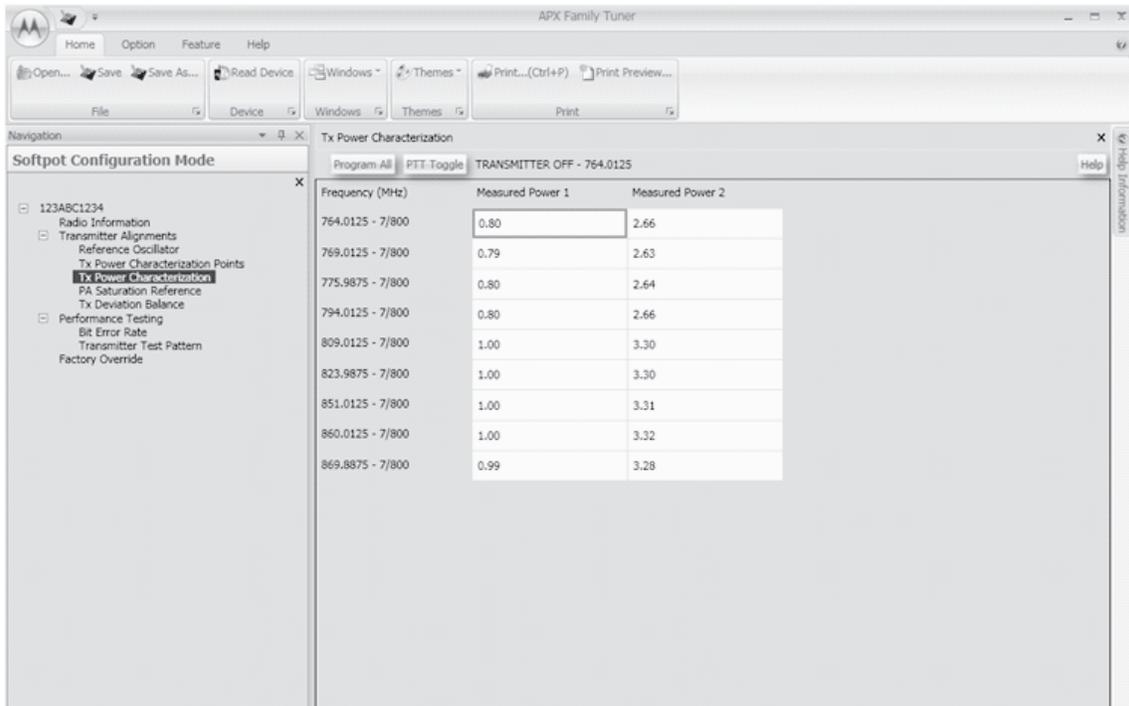
Figure 6-18. Transmit Power Characterization Alignment Screen (700/800 MHz)
