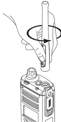
Figure 8-4. Removing the Antenna
