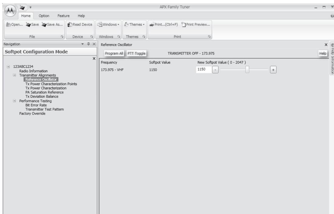
Figure 6-5. Reference Oscillator Alignment Screen (VHF)
