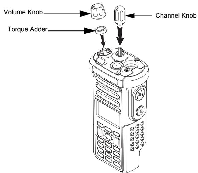
Figure 8-47. Reassemble the Volume Knob and Channel Knob
