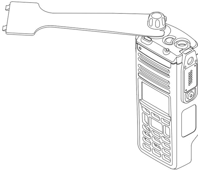
Figure 7-5. Removing the Multi Function Knob
