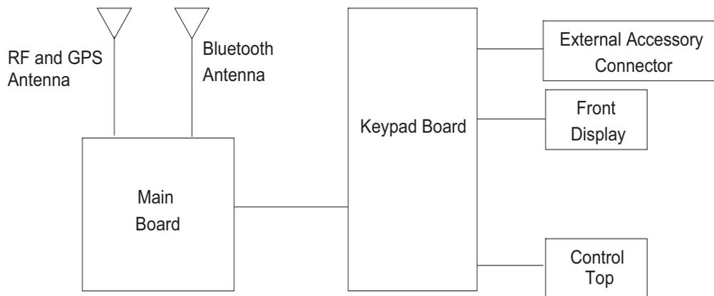
Figure 3-1. APX 2000/ APX 4000 (Two Knobs) Overall Block Diagram
