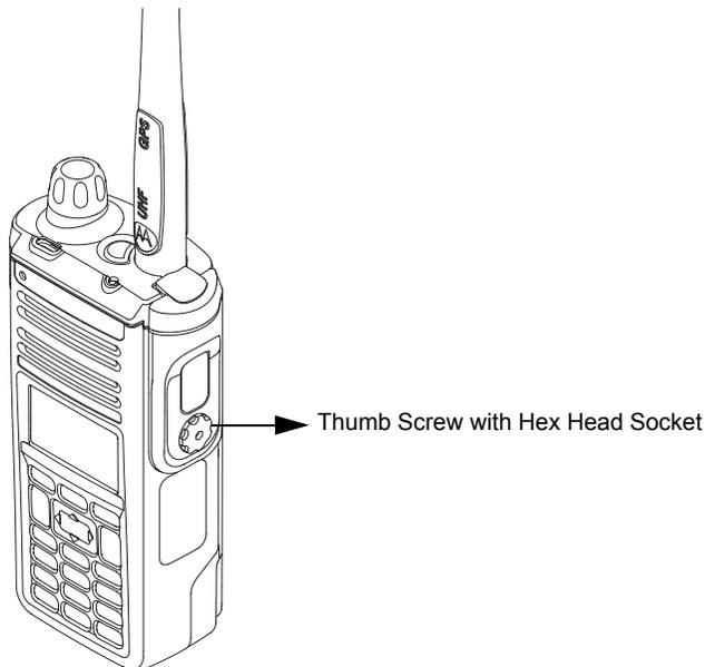
Figure 7-37. Securing the Cover
