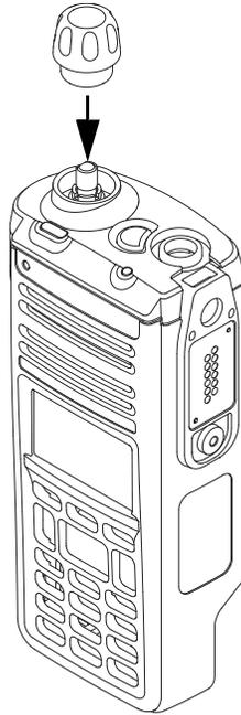
Figure 7-40. Reassemble the Multi Function Knob
