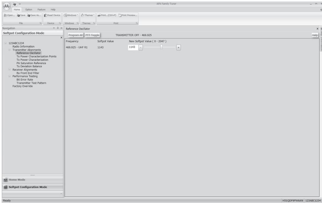
Figure 6-6. Reference Oscillator Alignment Screen (UHF1)
