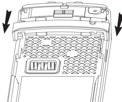
Figure 7-14. Remove the Shroud
