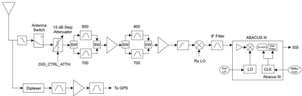
Figure 3-4. Receiver Block Diagram (700/800 MHz)
