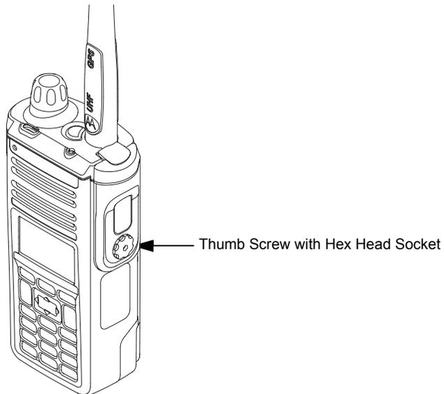
Figure 8-6. Removing the Thumb Screw
