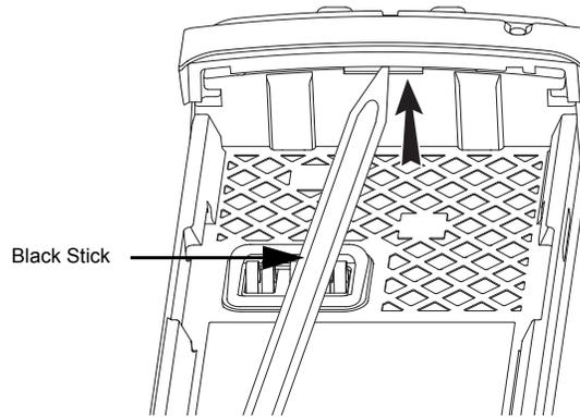
Figure 7-13. Disengage the Shroud
