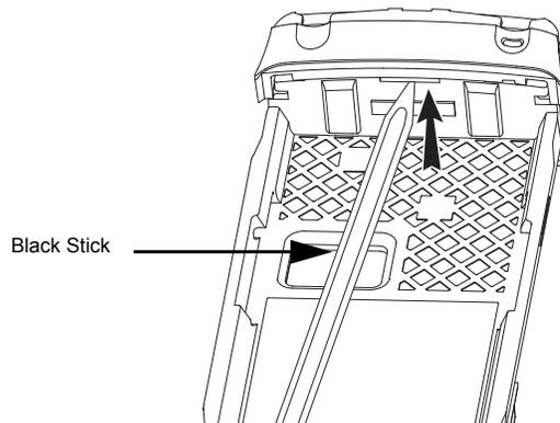
Figure 8-17. Disengage the Shroud
