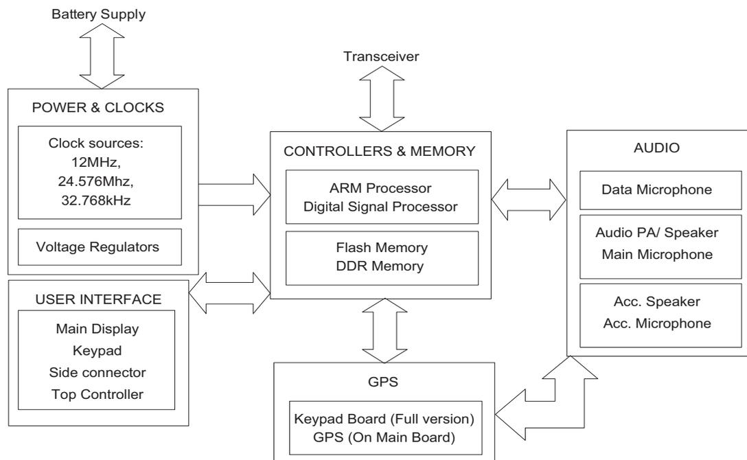
Figure 3-7. Controller Block Diagram
