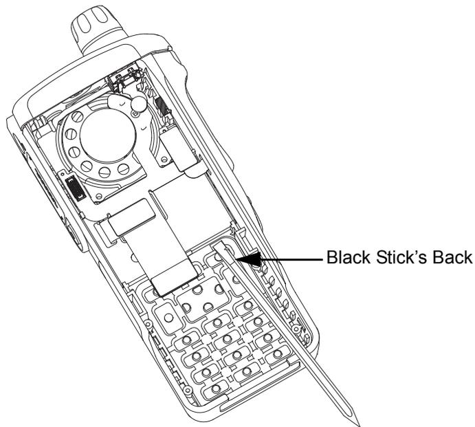
*Figure 8-30. Assemble the Keypad*
