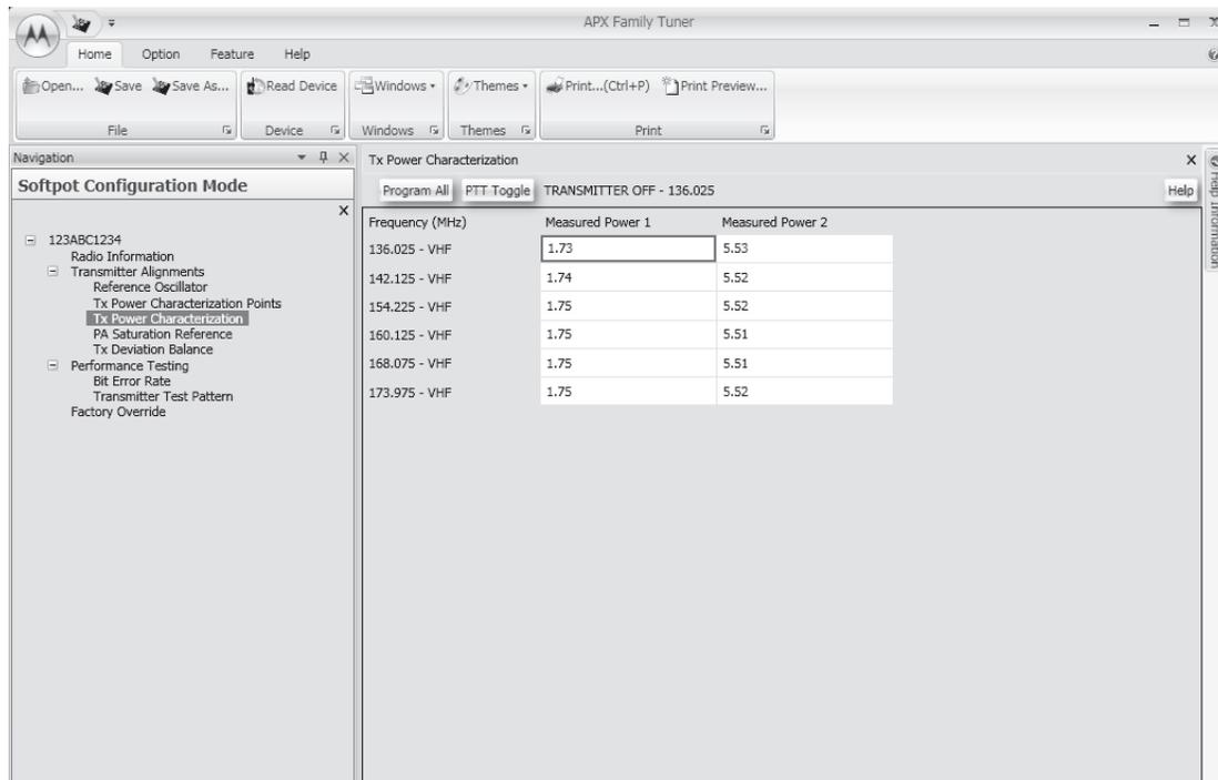
Figure 6-15. Transmit Power Characterization Alignment Screen (VHF)
