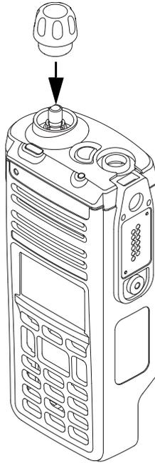
Figure 7-38. Reassemble the Multi Function Knob
