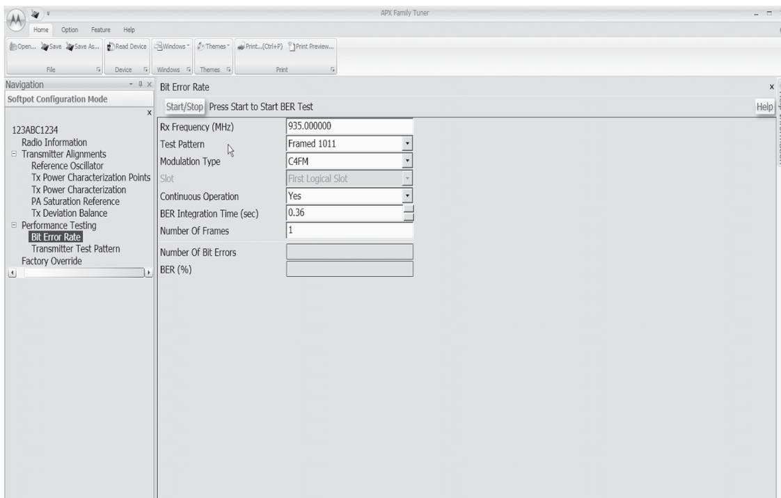
Figure 6-10. Bit Error Rate Screen (900 MHz)
