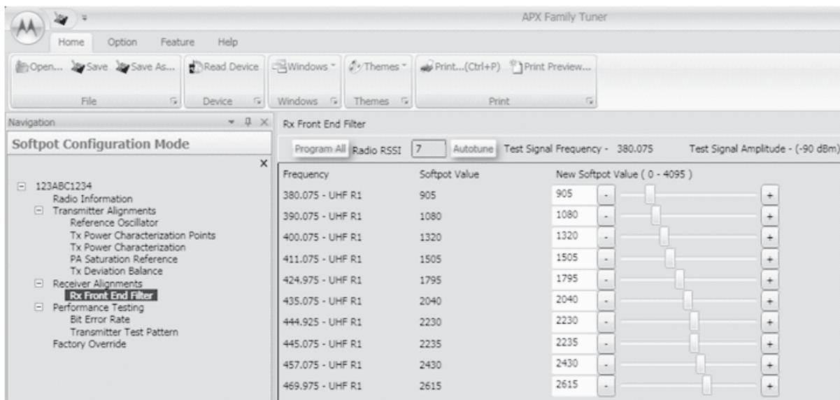
Figure 6-25. Front End Filter Alignment Screen (UHF1)
