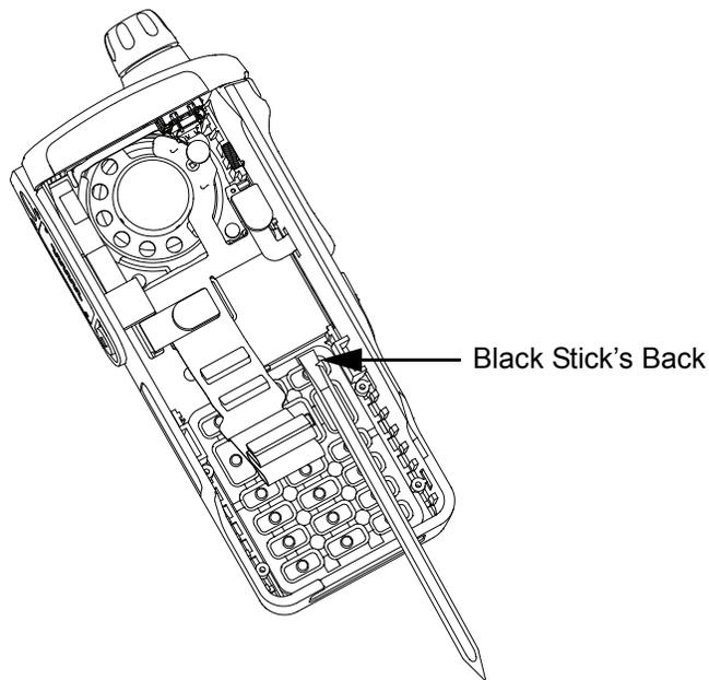
*Figure 7-25. Assemble the Keypad*
