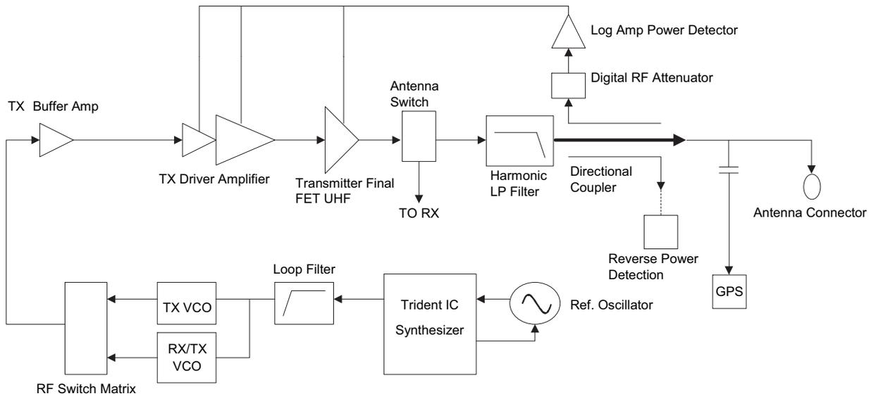
Figure 3-8. Transmitter (UHF1/UHF2) Block Diagram
