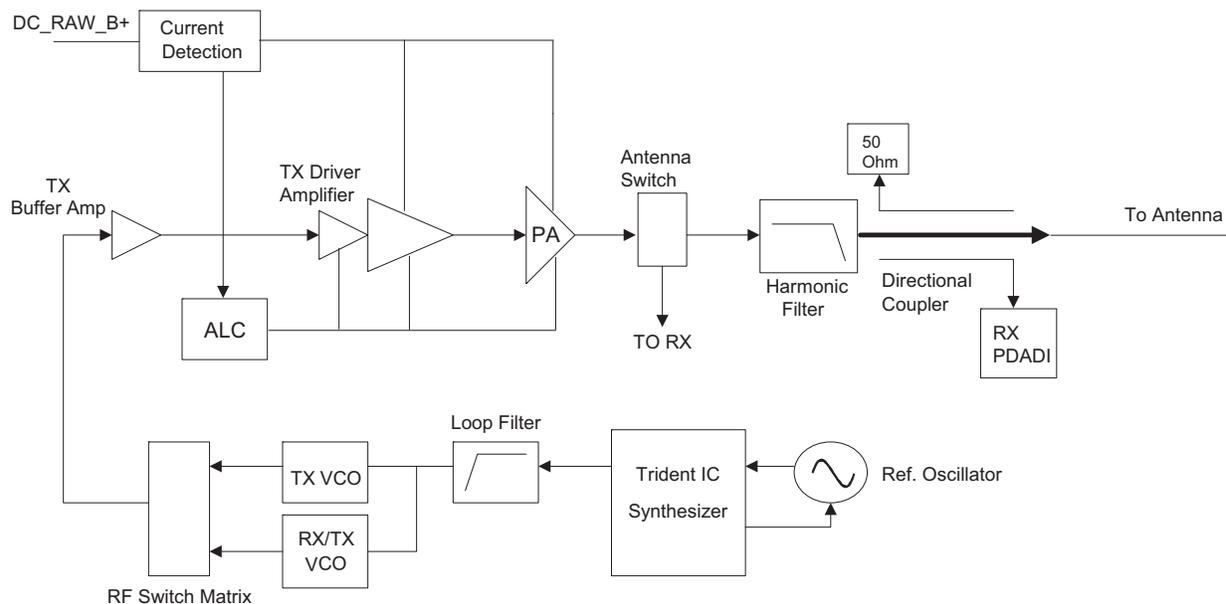
Figure 3-6. Transmitter Block Diagram
