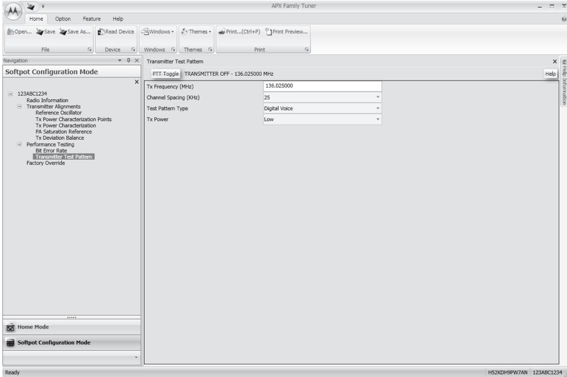
Figure 6-37. Transmitter Test Pattern Screen (VHF)
