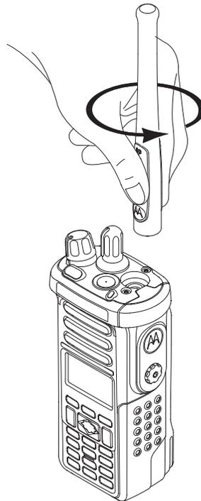
Figure 8-4. Removing the Antenna
