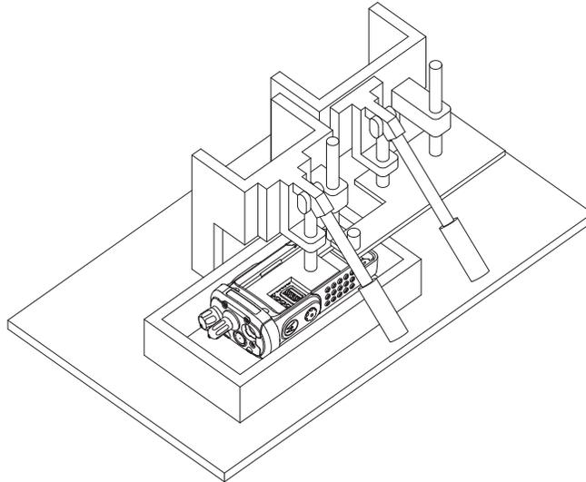
Figure 8-55. Attaching Vacuum Test Fixture
