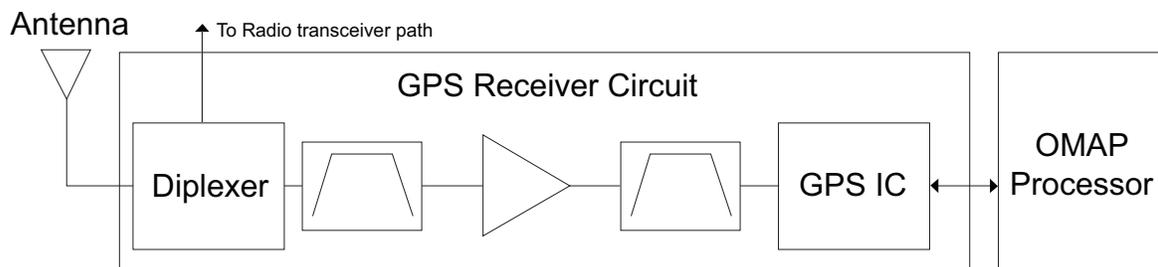
Figure 3-3. GPS Diagram
