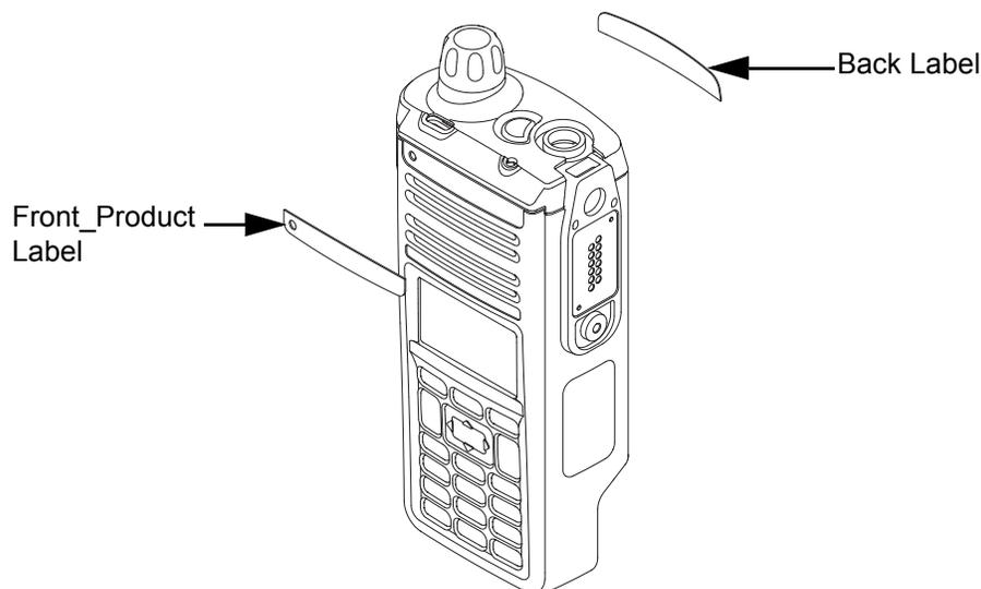
Figure 7-23. Serviceable Components – Main Housing
