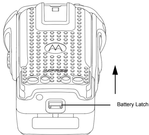
Figure 8-2. Lifting up the latch
