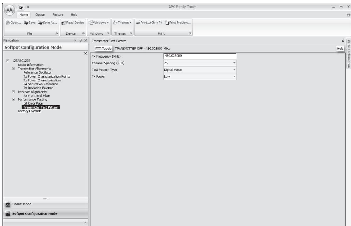
Figure 6-29. Transmitter Test Pattern Screen (UHF2)
