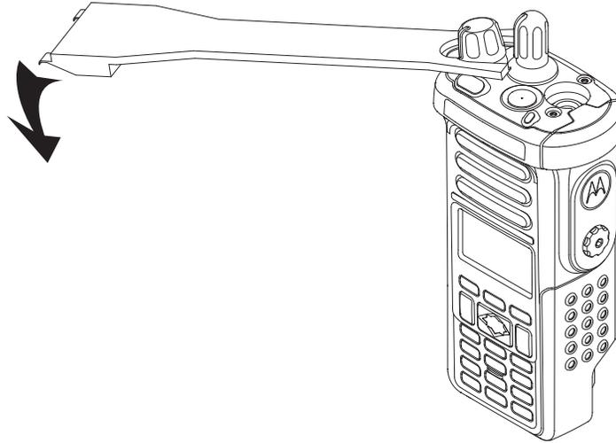
Figure 8-5. Removing the Volume Knob
