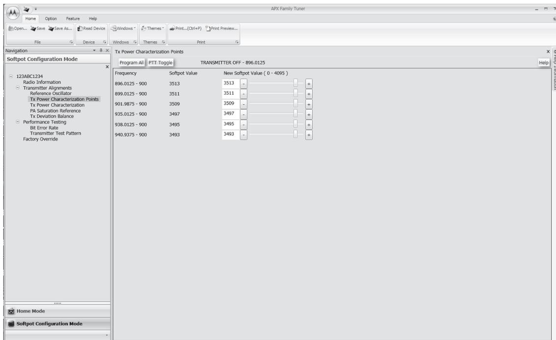
Figure 6-14. Transmit Power Characterization Points Alignment Screen (900 MHz)
