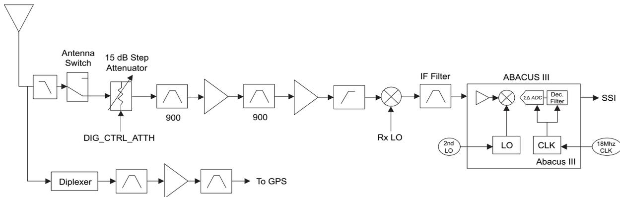
Figure 3-5. Receiver Block Diagram (900 MHz)
