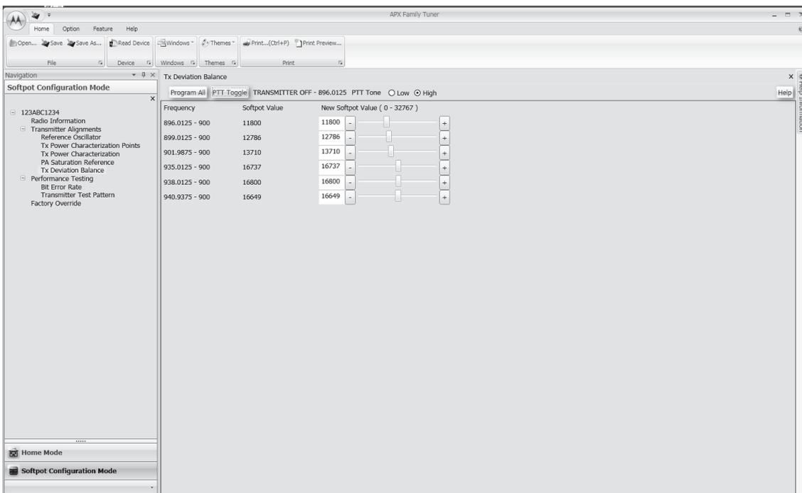
Figure 6-29. Transmit Deviation Balance Alignment Screen (900 MHz)
