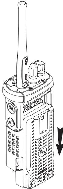
Figure 8-3. Removing the Battery
