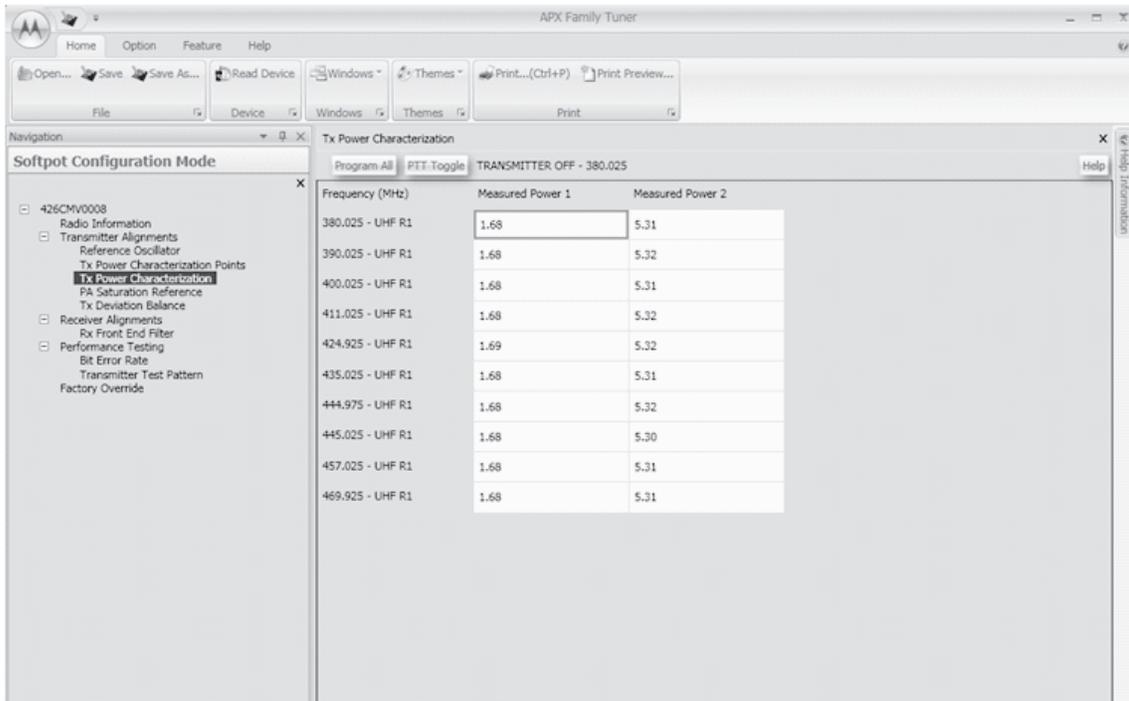
Figure 6-16. Transmit Power Characterization Alignment Screen (UHF1)
