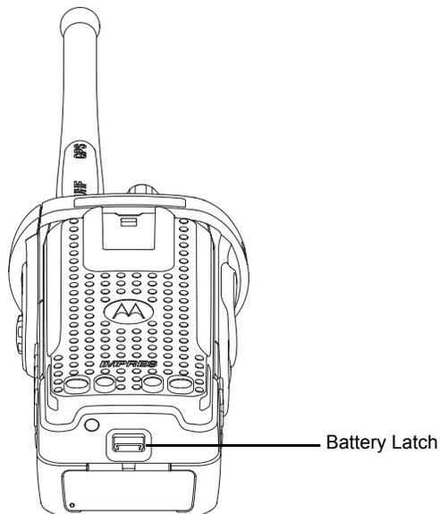
Figure 8-2. Lifting up the latch
