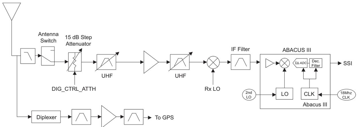
Figure 3-3. Receiver Block Diagram (UHF1/UHF2)
