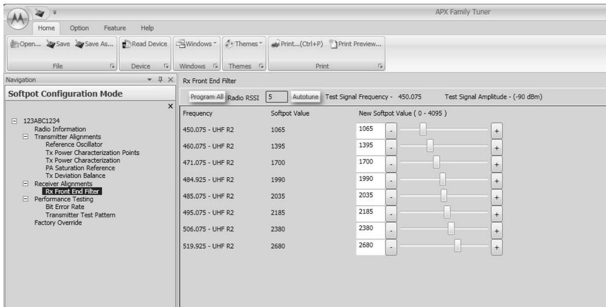
Figure 6-31. Front End Filter Alignment Screen (UHF2)
