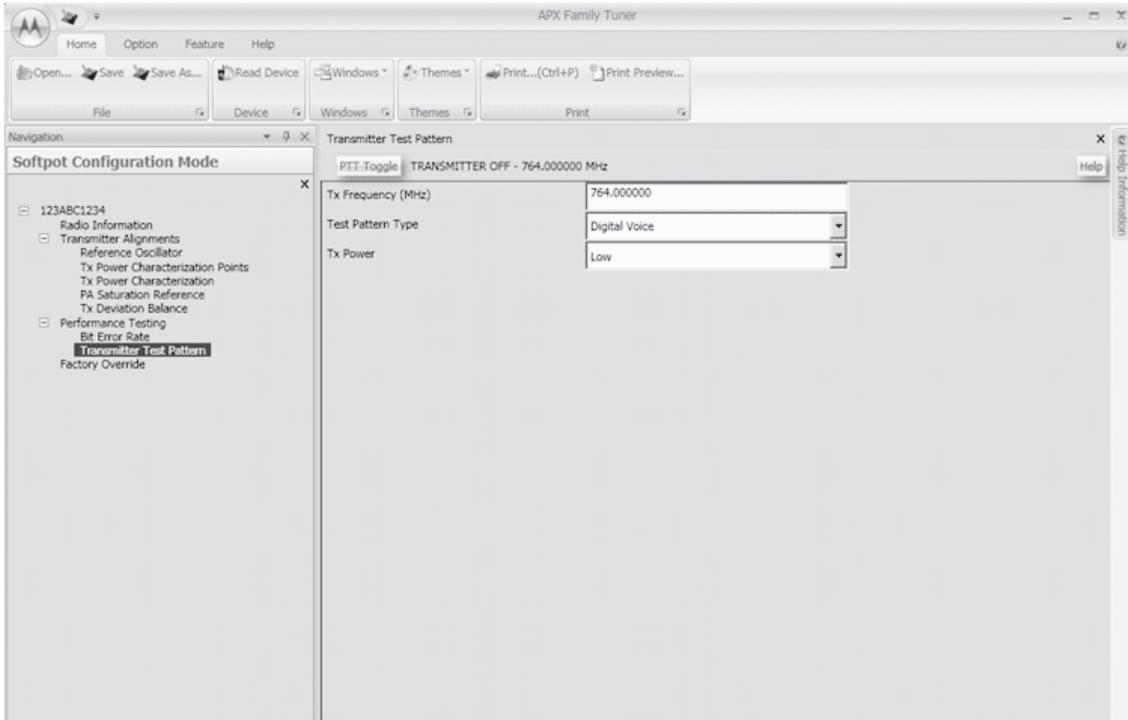
Figure 6-30. Transmitter Test Pattern Screen (700/800 MHz)
