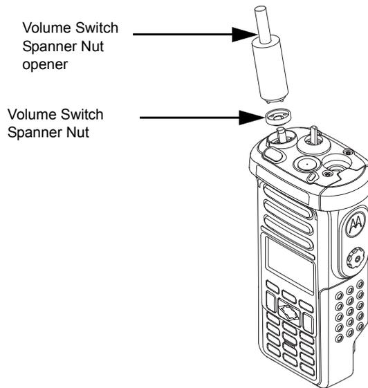
Figure 8-9. Removing the Volume Switch Spanner Nut
