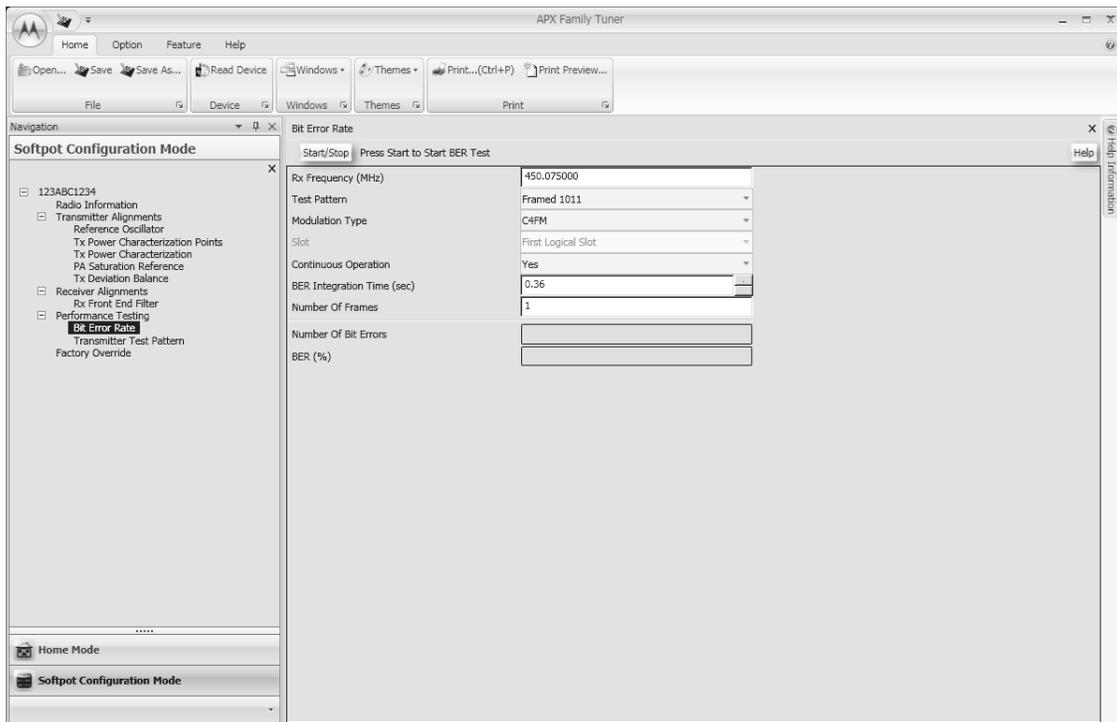
Figure 6-25. Bit Error Rate Screen (UHF2)
