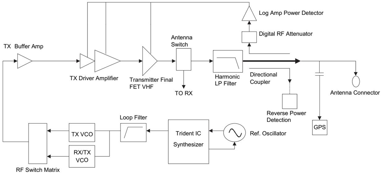
Figure 3-7. Transmitter (VHF) Block Diagram
