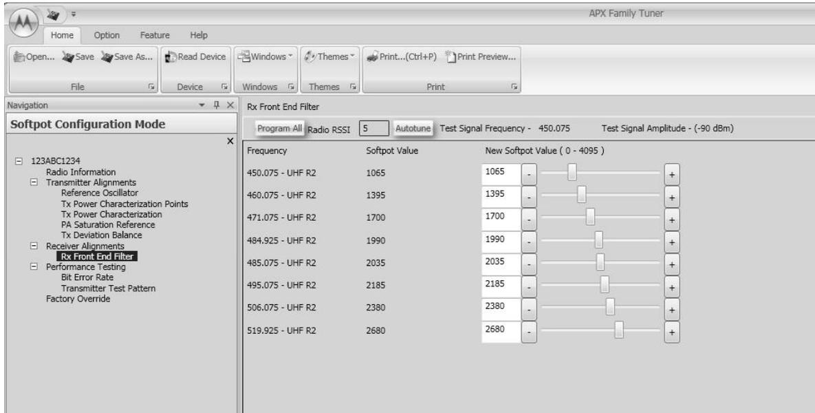
Figure 6-22. Front End Filter Alignment Screen (UHF2)
