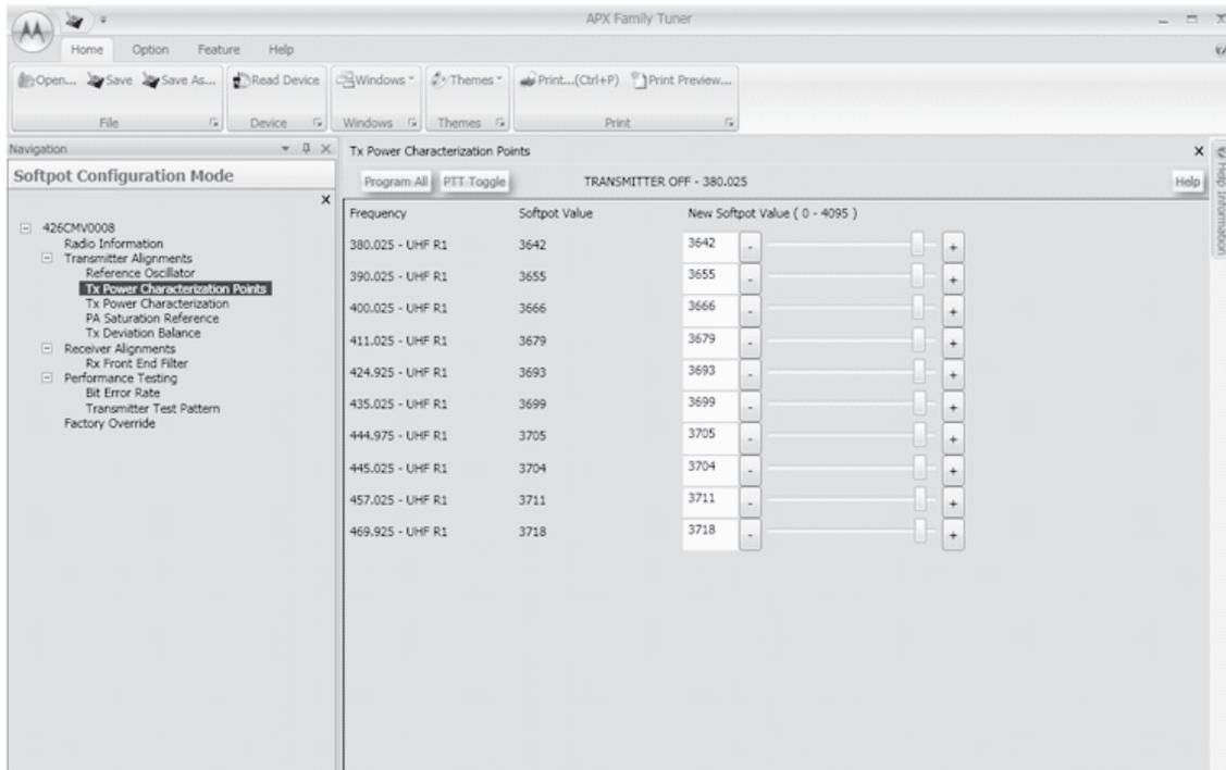
Figure 6-11. Transmit Power Characterization Points Alignment Screen (UHF1)
