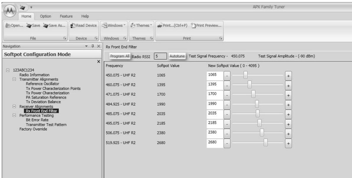
Figure 6-26. Front End Filter Alignment Screen (UHF2)
