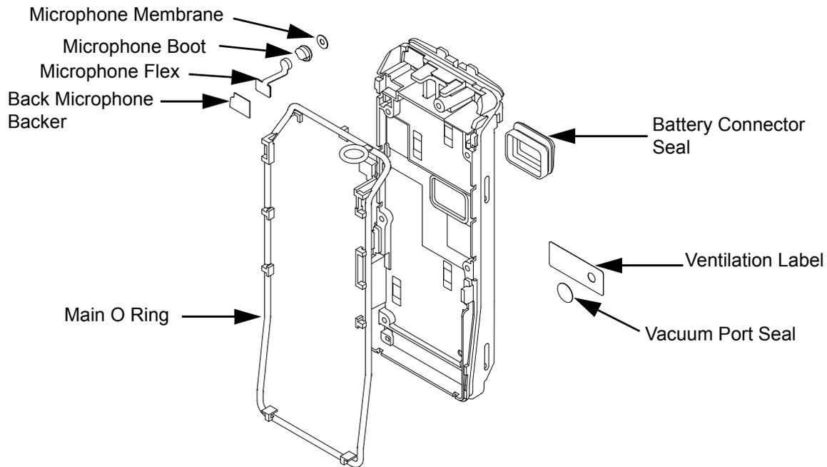
Figure 7-22. Serviceable Components – Chassis Assembly
