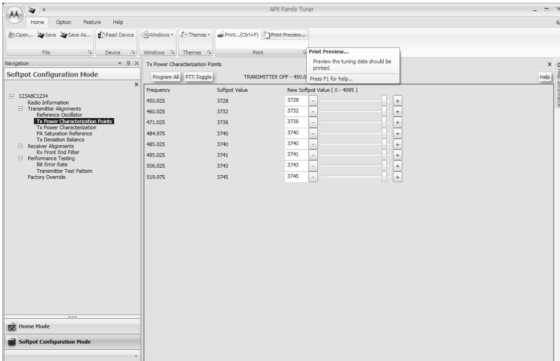
Figure 6-12. Transmit Power Characterization Points Alignment Screen (UHF2)
