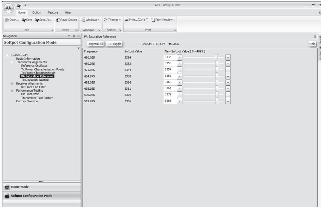
Figure 6-22. PA Saturation Referencing Alignment Screen (UHF2)
