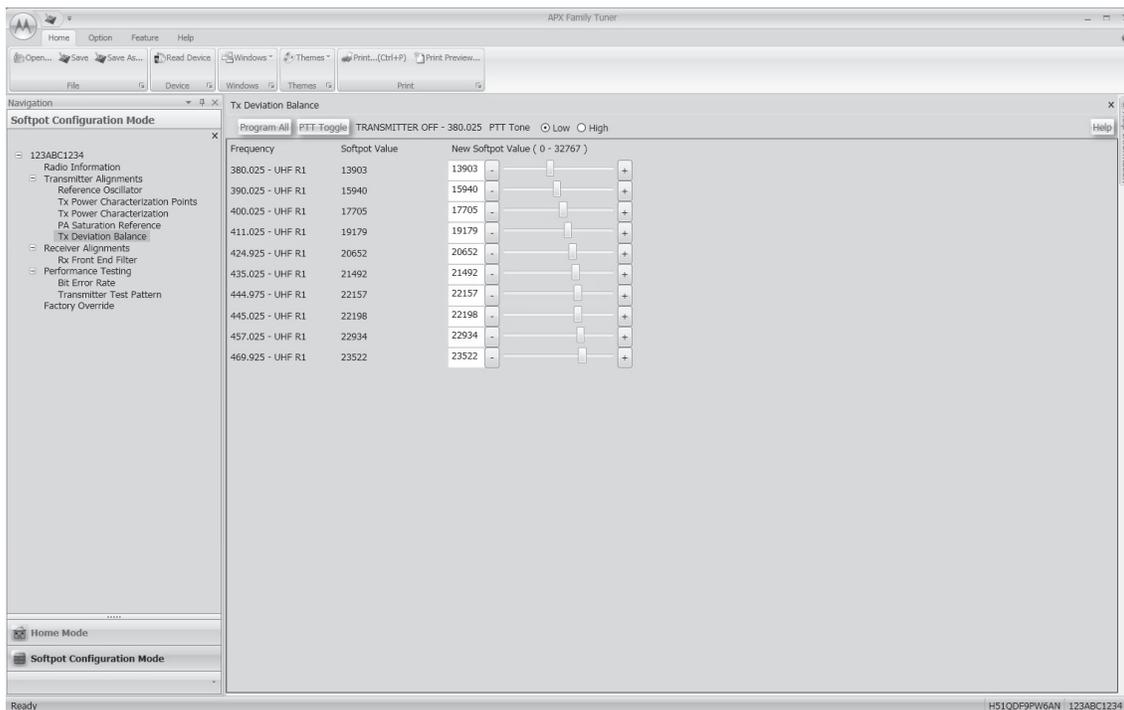
Figure 6-18. Transmit Deviation Balance Alignment Screen (UHF1)
