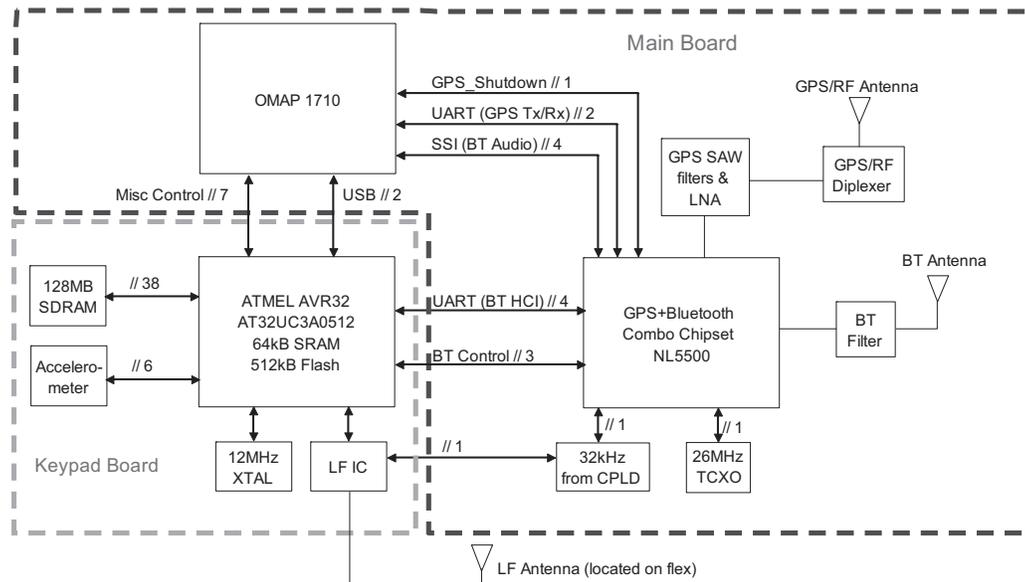
Figure 3-10. GPS/Bluetooth/Accelerometer Block Diagram
