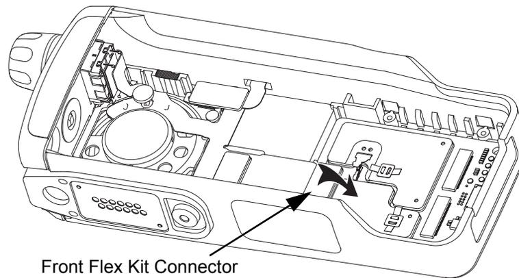
*Figure 8-31. Plug in the Front Kit Flex Connector*
