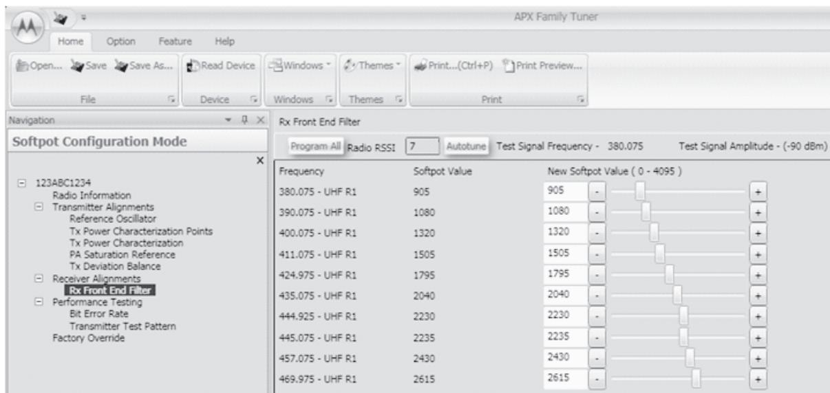
Figure 6-21. Front End Filter Alignment Screen (UHF1)
