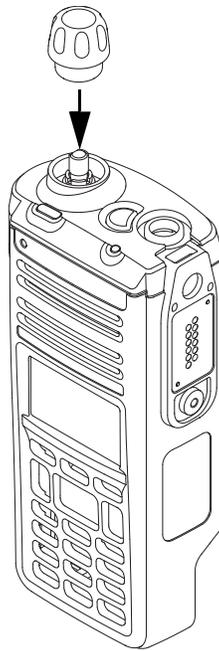
Figure 8-40. Reassemble the Multi Function Knob
