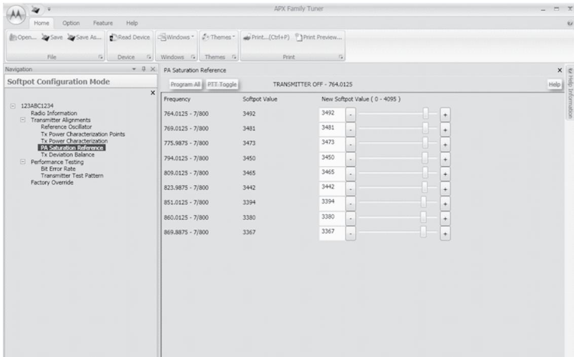
Figure 6-23. PA Saturation Referencing Alignment Screen (700/800 MHz)
