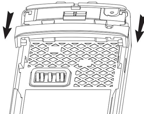
Figure 7-15. Remove the Shroud
