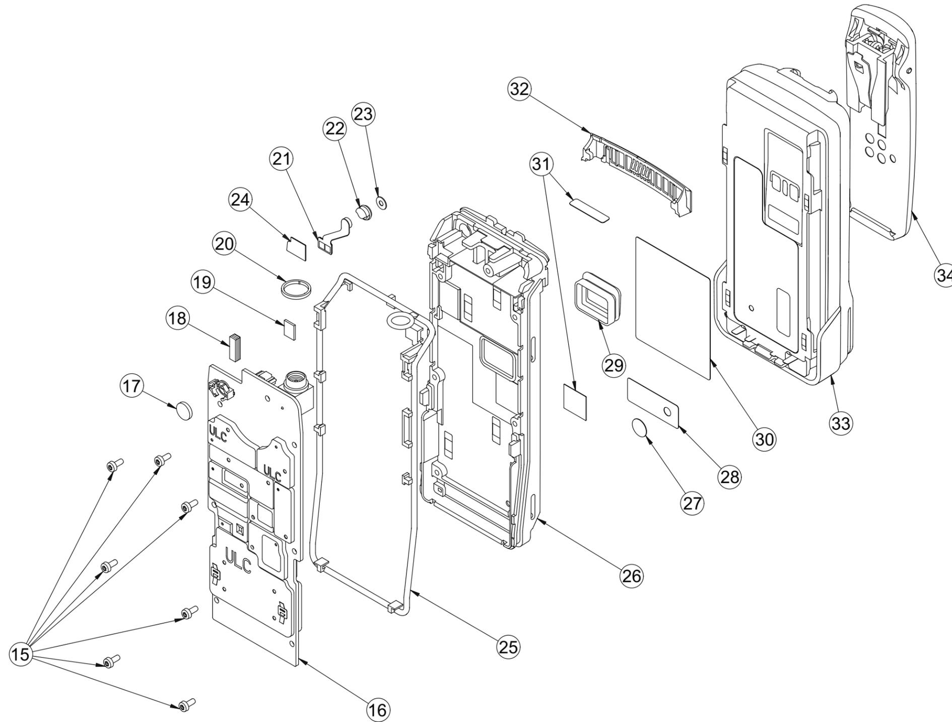
Figure 9-2. APX 1000 Back Kit Exploded View
