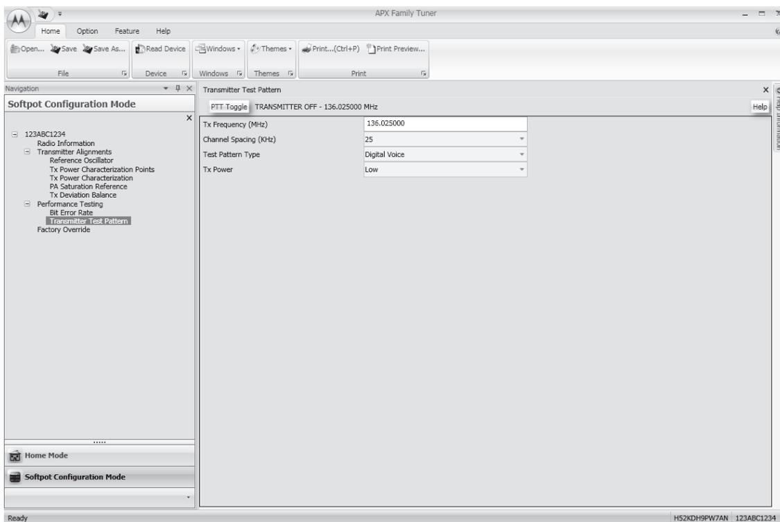
Figure 6-31. Transmitter Test Pattern Screen (VHF)
