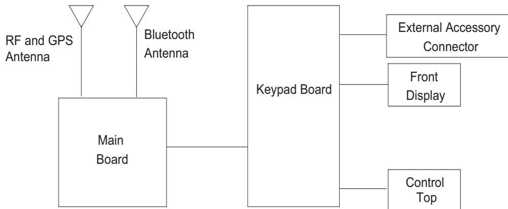
Figure 3-1. APX 1000 Overall Block Diagram
