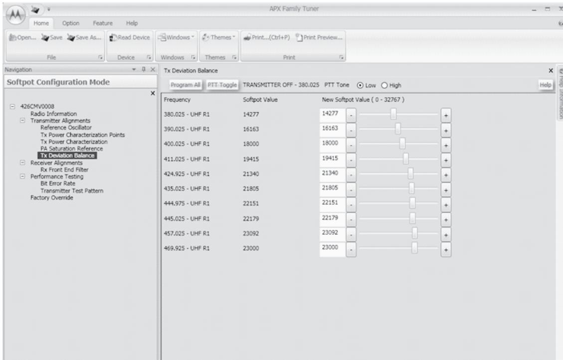
Figure 6-26. Transmit Deviation Balance Alignment Screen (UHF1)
