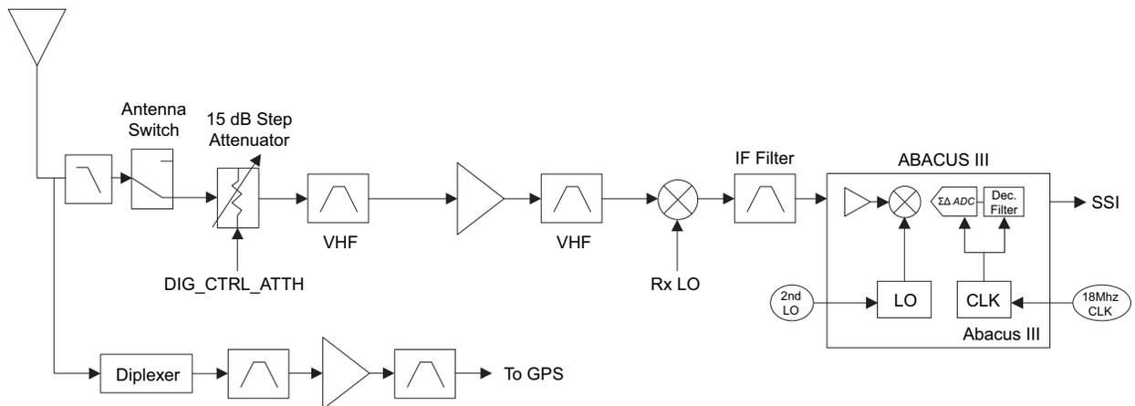
Figure 3-2. Receiver Block Diagram (VHF)
