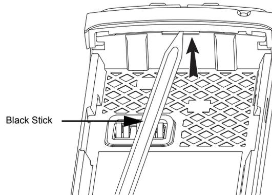
Figure 8-14. Disengage the Shroud
