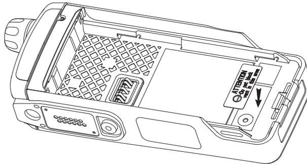
*Figure 7-41. Assemble the Ventilation Label*
