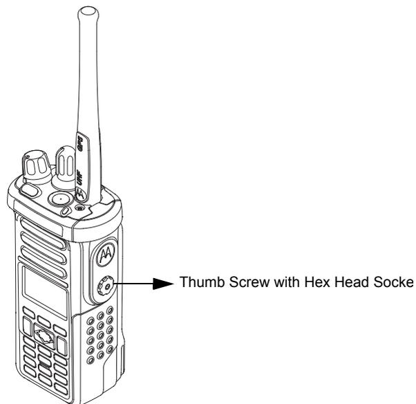
Figure 8-49. Securing the Cover
