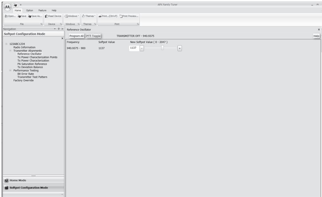
Figure 6-5. Reference Oscillator Alignment Screen (900 MHz)
