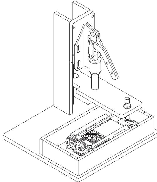
Figure 8-46. Attaching Vacuum Test Fixture
