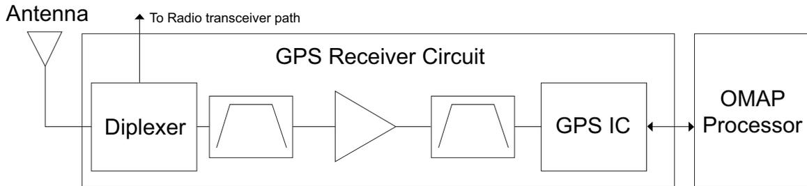
Figure 3-5. GPS Diagram
