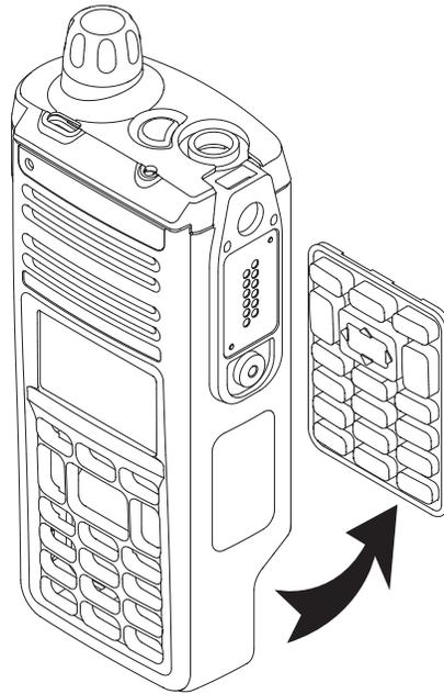
Figure 7-20. Remove the Keypad
