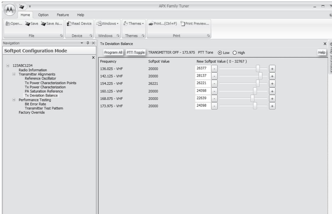
Figure 6-21. Transmit Deviation Balance Alignment Screen (VHF)
