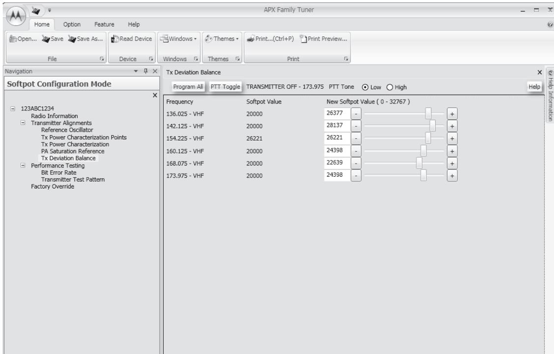
Figure 6-25. Transmit Deviation Balance Alignment Screen (VHF)
