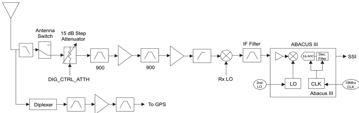
Figure 3-2. Receiver Block Diagram (900 MHz)
