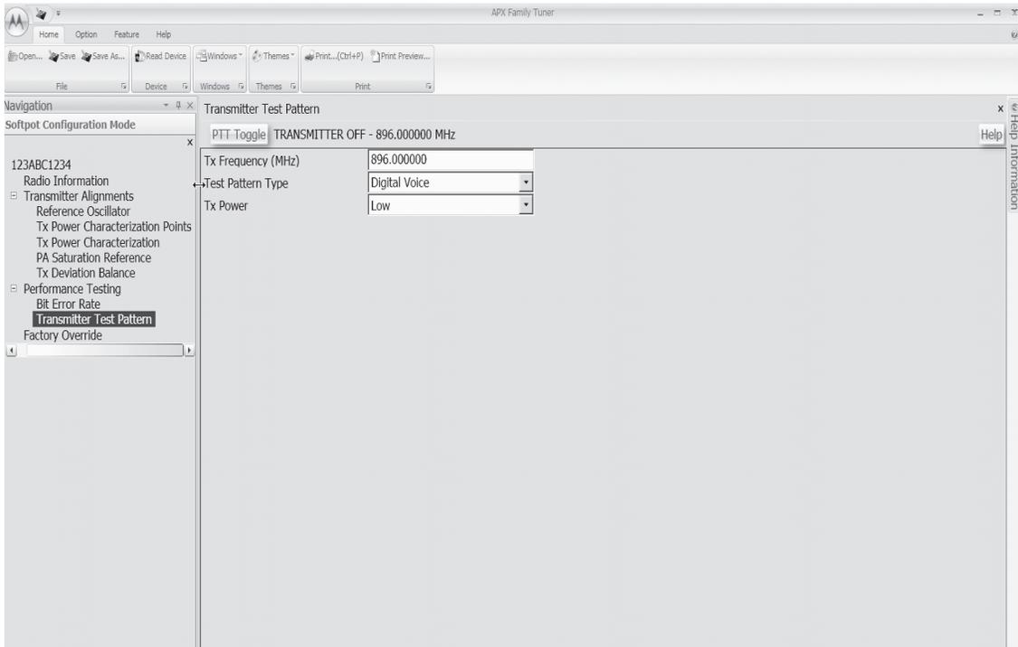
Figure 6-41. Transmitter Test Pattern Screen (900 MHz)
