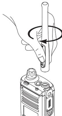
Figure 7-41. Attaching the Antenna
