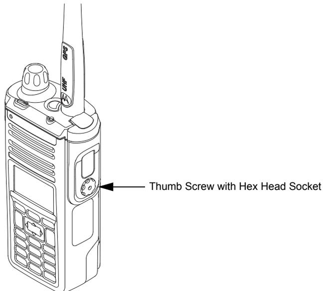
Figure 7-39. Securing the Cover
