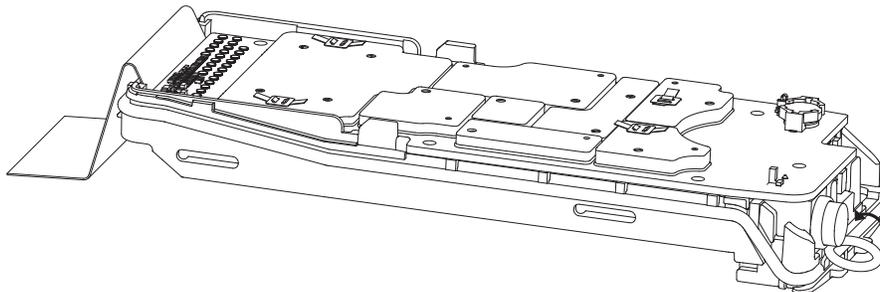
*Figure 8-34. Assemble the Main O-Ring at Antenna Holder*
