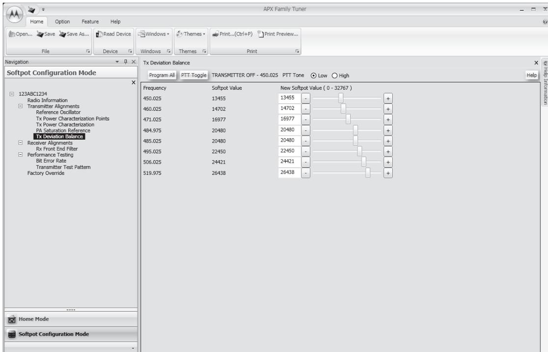
Figure 6-23. Transmit Deviation Balance Alignment Screen (UHF2)
