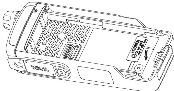
Figure 8-43. Assemble the Ventilation Label
