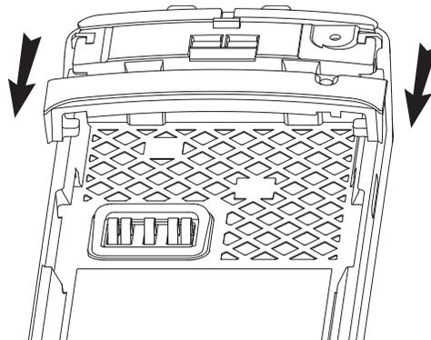
Figure 8-15. Remove the Shroud
