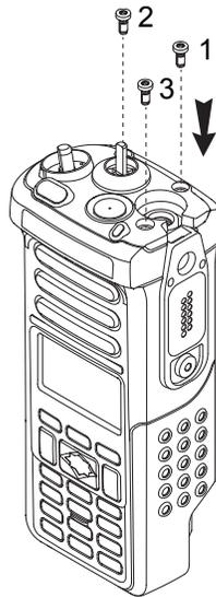
Figure 8-45. Tighten the Screws
