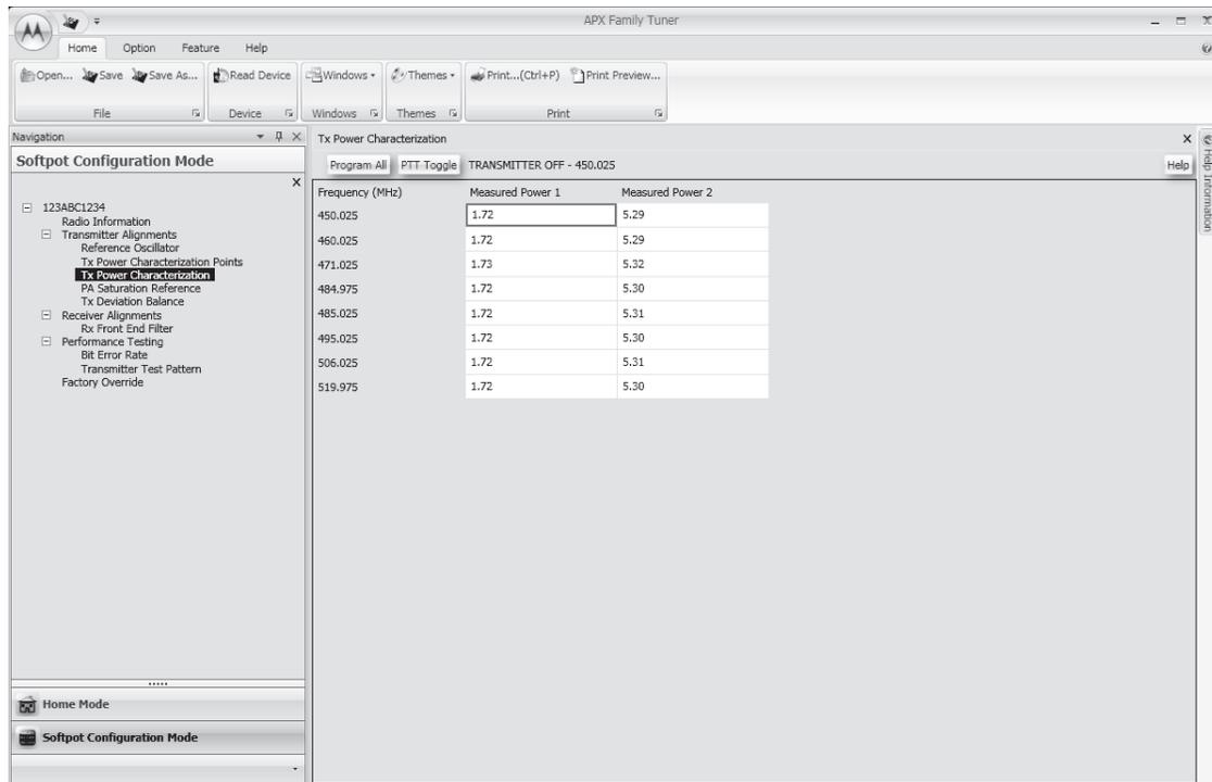
Figure 6-17. Transmit Power Characterization Alignment Screen (UHF2)
