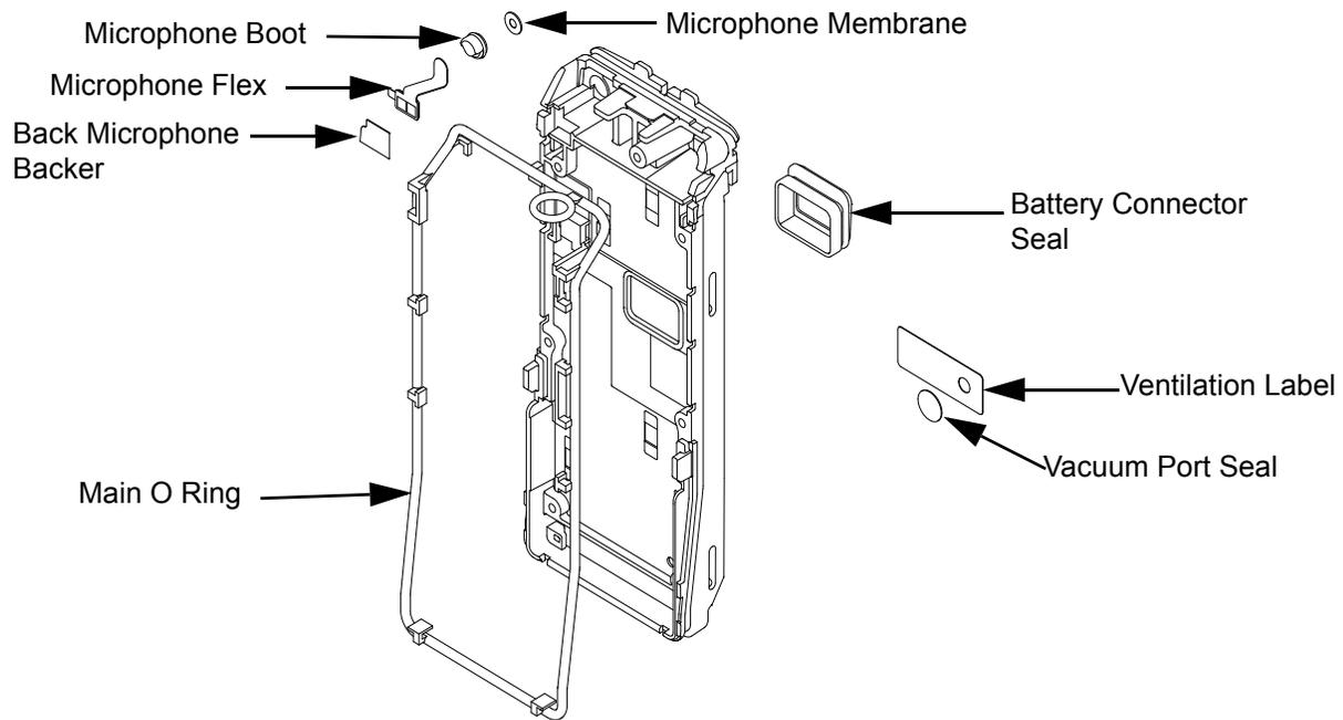
Figure 7-23. Serviceable Components – Chassis Assembly
