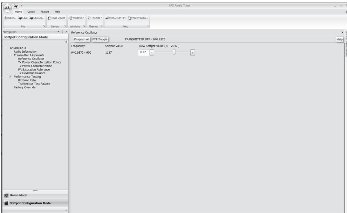
Figure 6-9. Reference Oscillator Alignment Screen (900 MHz)
