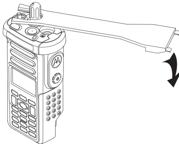
Figure 8-6. Removing the Channel Knob
