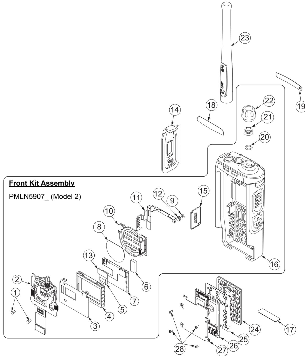
Figure 9-1. APX 1000 Front Kit Exploded View
