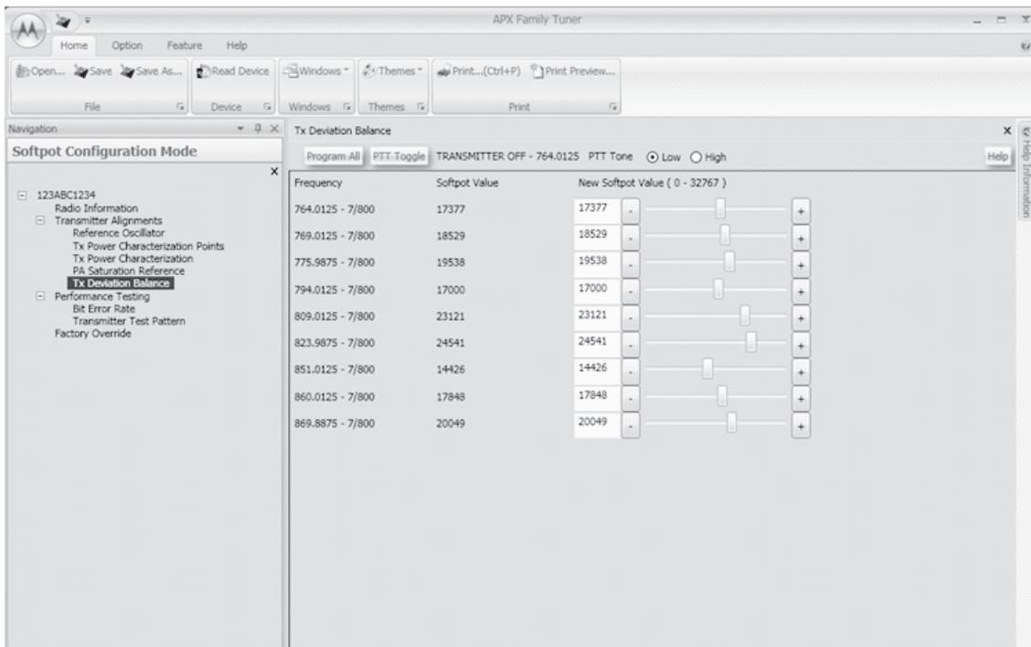
Figure 6-28. Transmit Deviation Balance Alignment Screen (700/800 MHz)
