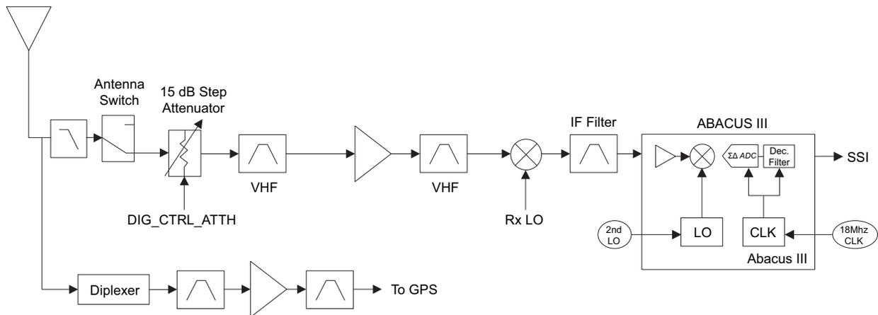
Figure 3-2. Receiver Block Diagram (VHF)
