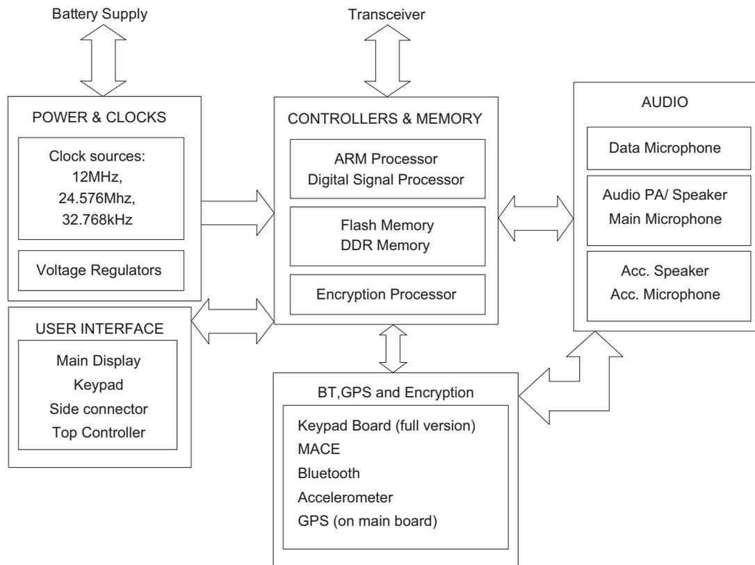
Figure 3-11. Controller Block Diagram
