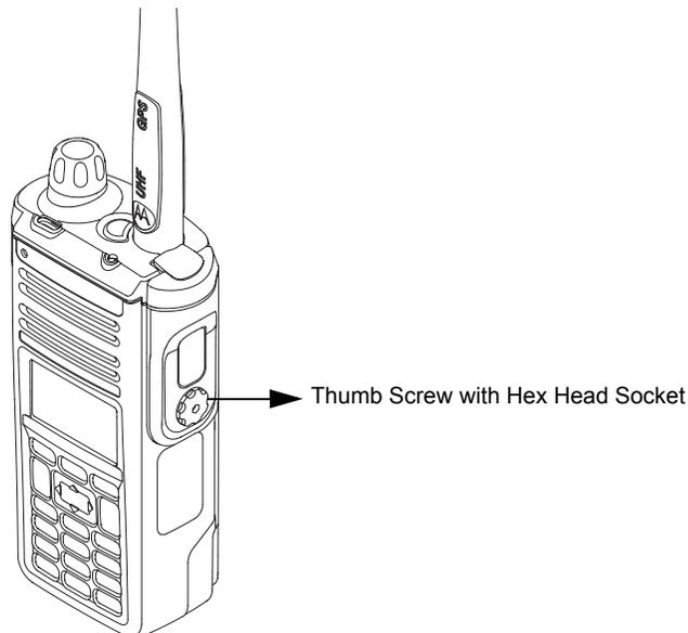
Figure 8-39. Securing the Cover
