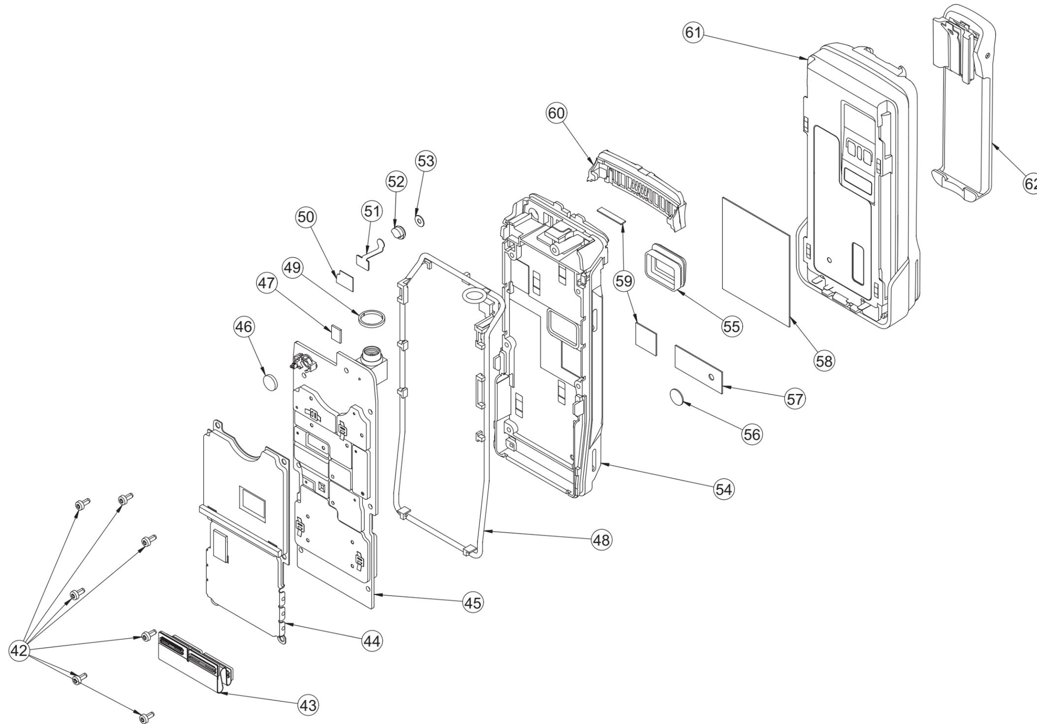
Figure 10-2. APX 2000/ APX 4000 (Two Knobs) Back Kit Exploded View
