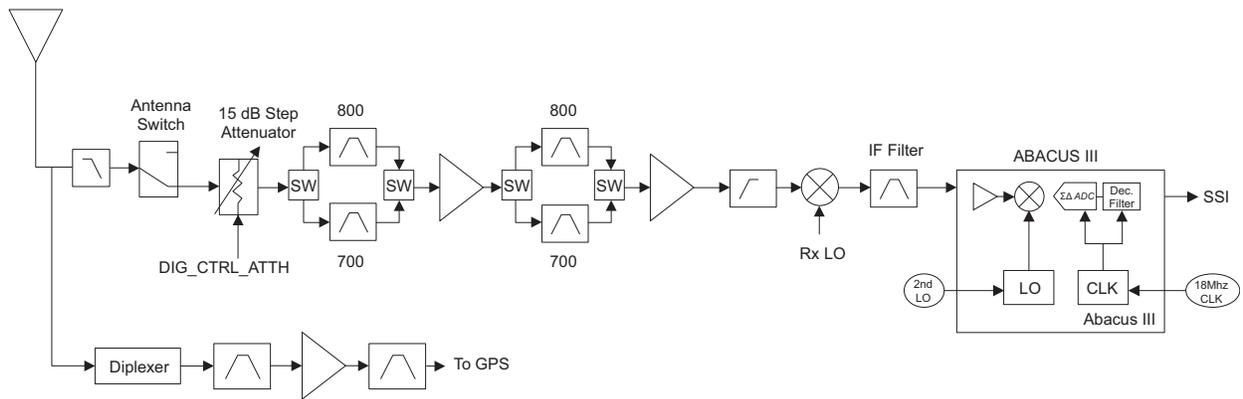
Figure 3-4. Receiver Block Diagram (700/800 MHz)
