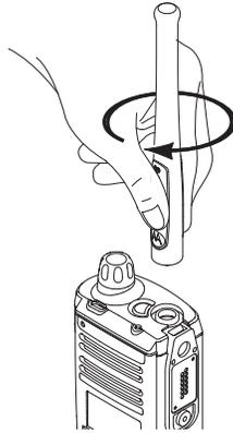
Figure 8-41. Attaching the Antenna
