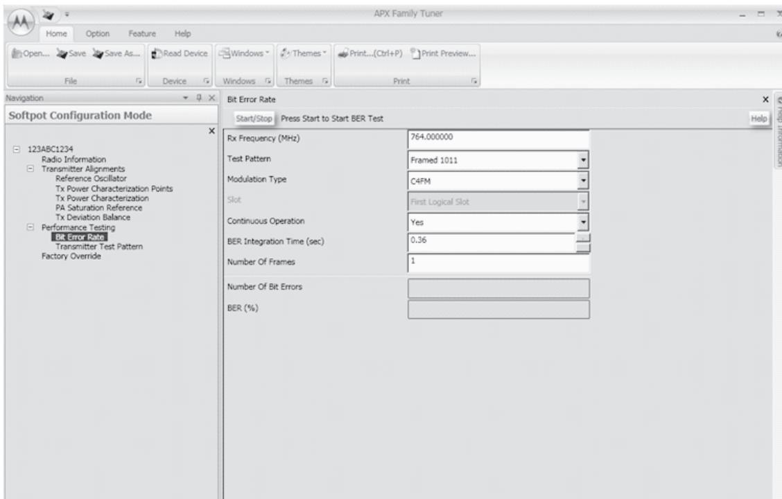
Figure 6-26. Bit Error Rate Screen (700/800 MHz)
