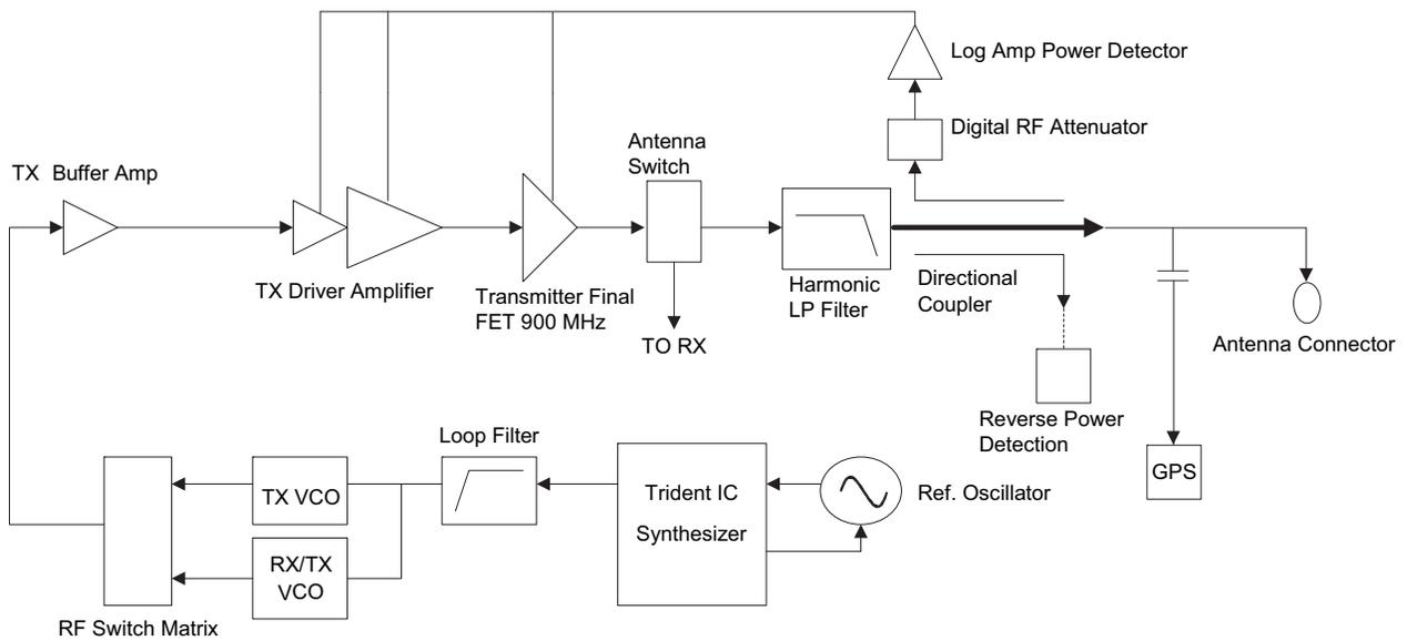
Figure 3-10. Transmitter (900 MHz) Block Diagram
