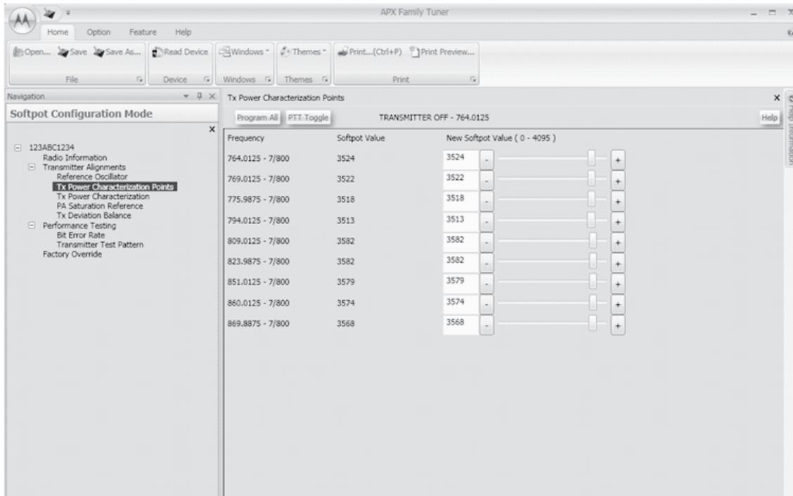
Figure 6-13. Transmit Power Characterization Points Alignment Screen (700/800 MHz)
