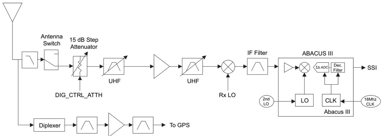
Figure 3-3. Receiver Block Diagram (UHF1/UHF2)
