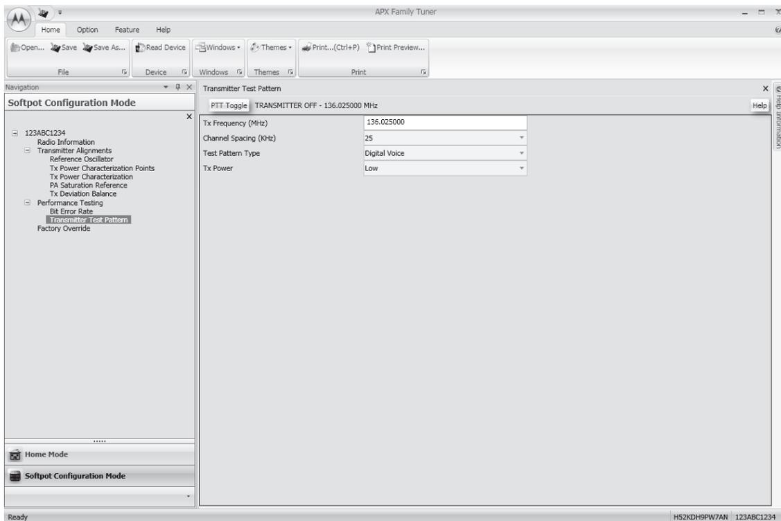
Figure 6-27. Transmitter Test Pattern Screen (VHF)
