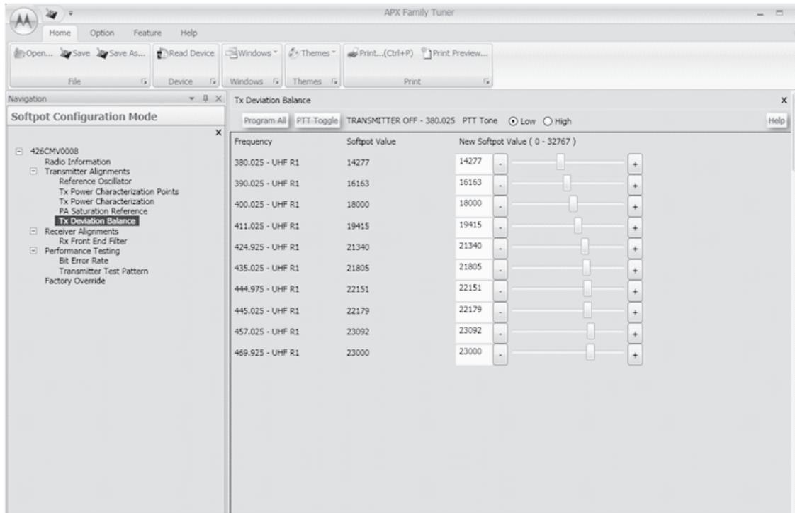
Figure 6-22. Transmit Deviation Balance Alignment Screen (UHF1)
