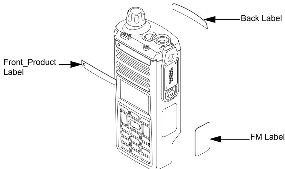
Figure 8-24. Serviceable Components – Main Housing
