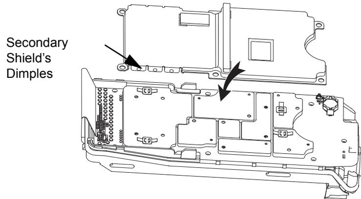
Figure 7-28. Assemble the Secondary Shield Assembly
