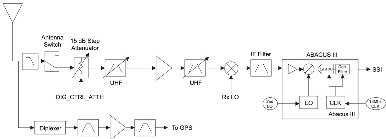
Figure 3-3. Receiver Block Diagram (UHF1/UHF2)
