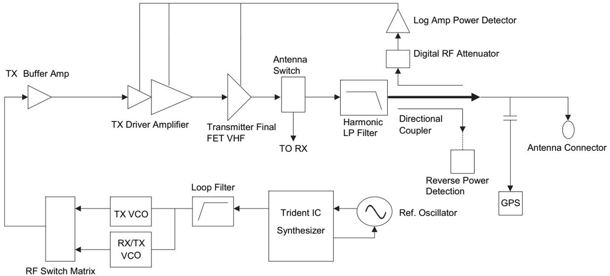
Figure 3-6. Transmitter (VHF) Block Diagram
