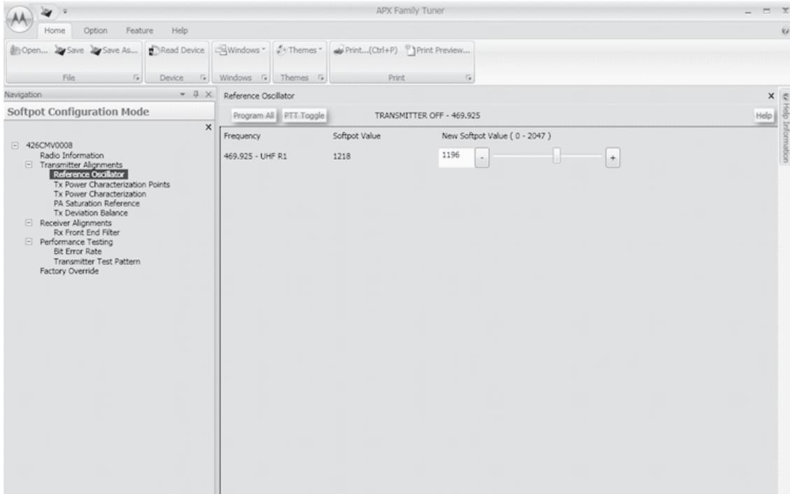
Figure 6-6. Reference Oscillator Alignment Screen (UHF1)
