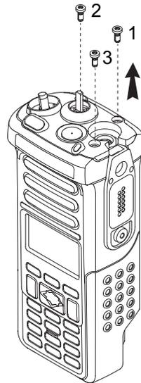
Figure 8-8. Unscrew the screws
