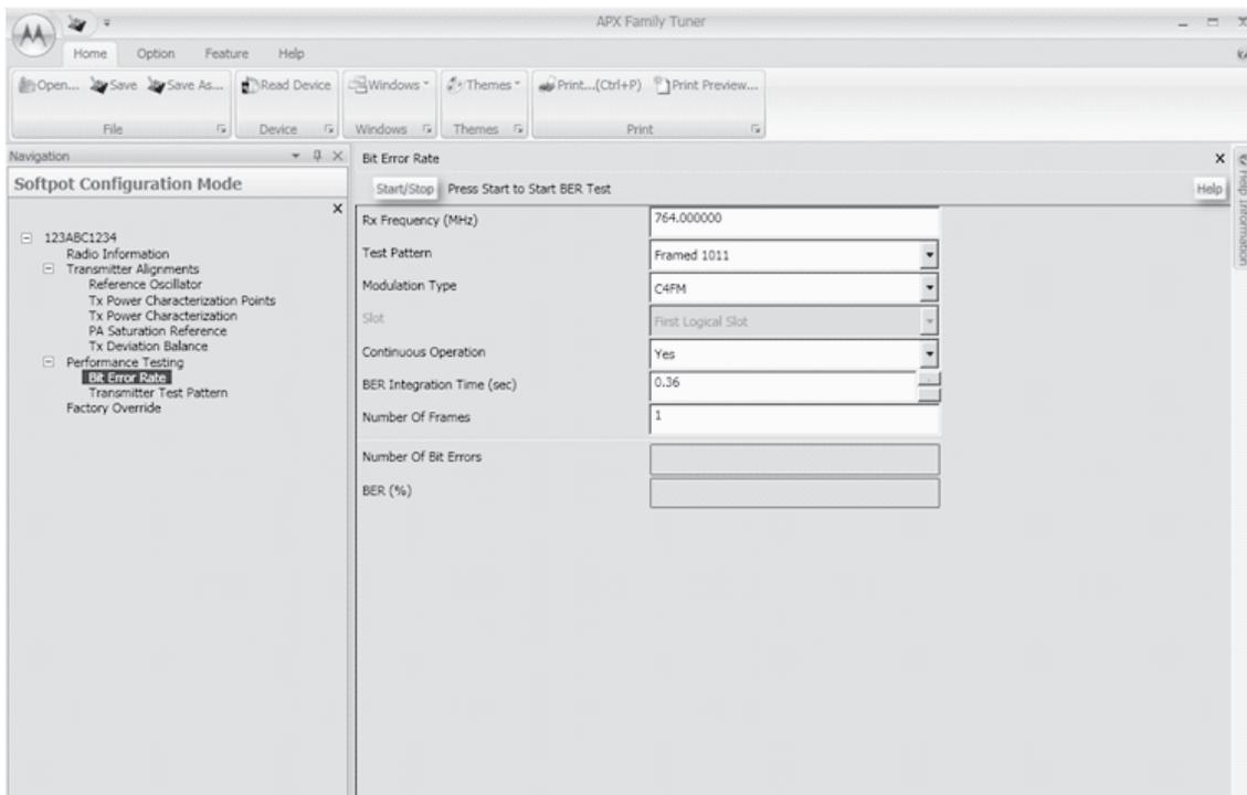
Figure 6-35. Bit Error Rate Screen (700/800 MHz)
