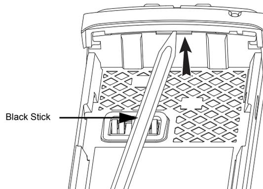
Figure 7-14. Disengage the Shroud
