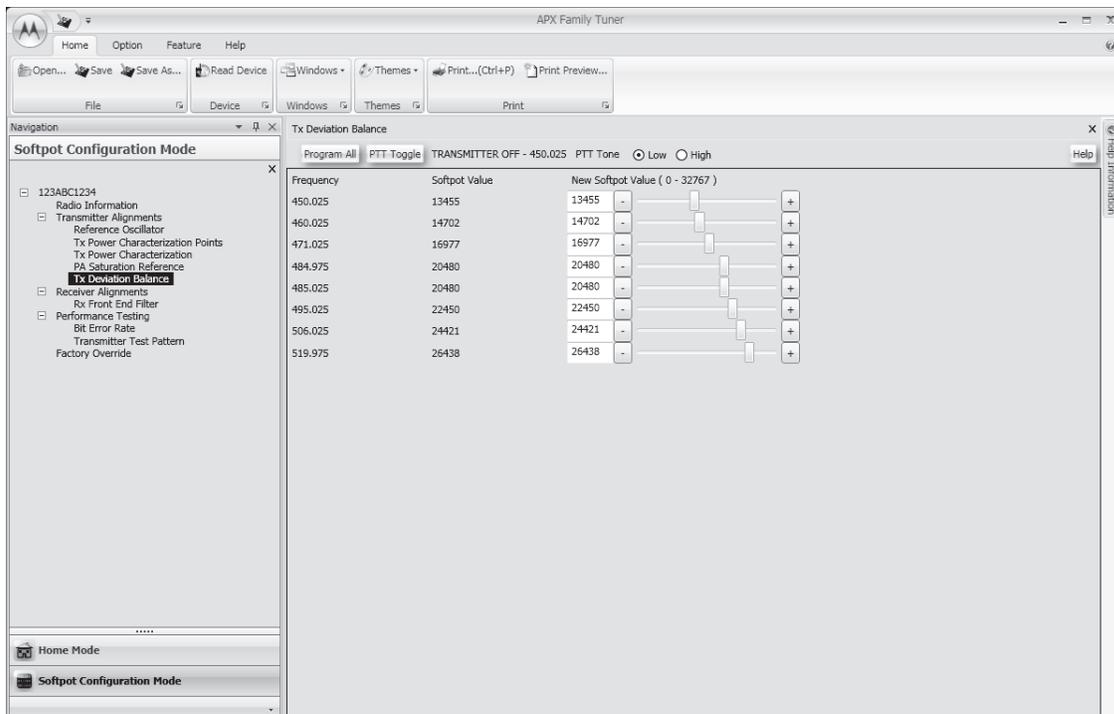
Figure 6-27. Transmit Deviation Balance Alignment Screen (UHF2)
