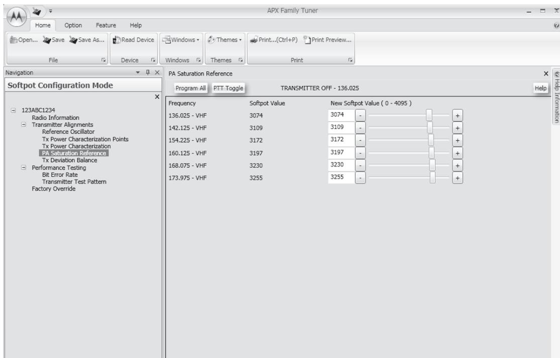
Figure 6-20. PA Saturation Referencing Alignment Screen (VHF)
