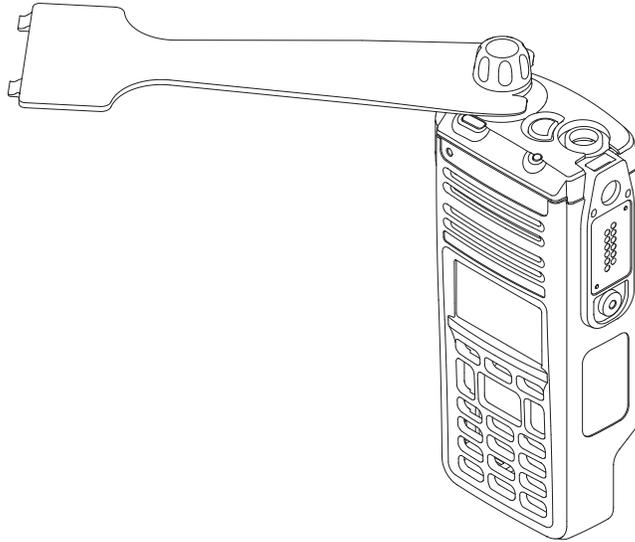
Figure 8-5. Removing the Multi Function Knob
