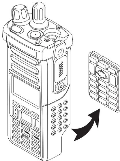
*Figure 8-24. Remove the Keypad*
