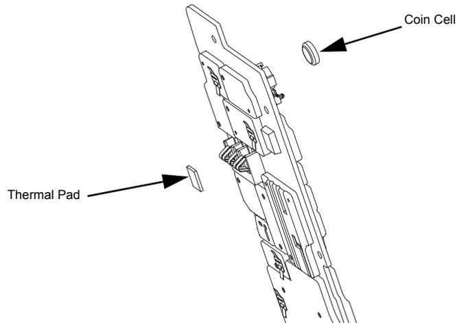
Figure 8-25. Serviceable Components – Main Board Assembly
