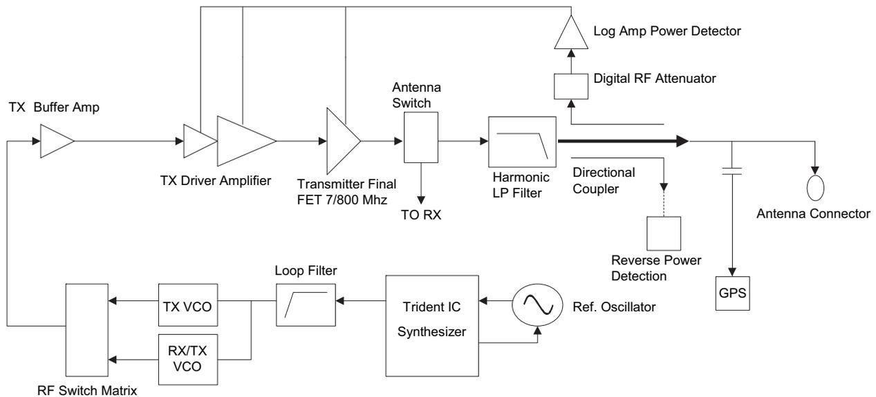
Figure 3-8. Transmitter (700/800 MHz) Block Diagram
