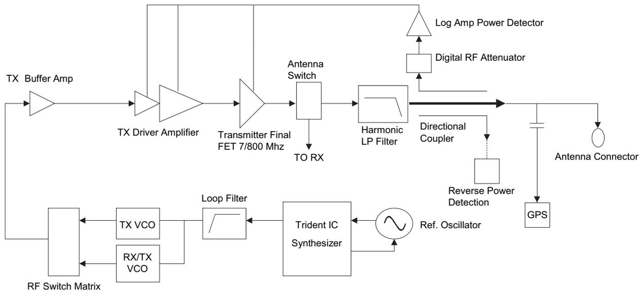
Figure 3-9. Transmitter (700/800 MHz) Block Diagram
