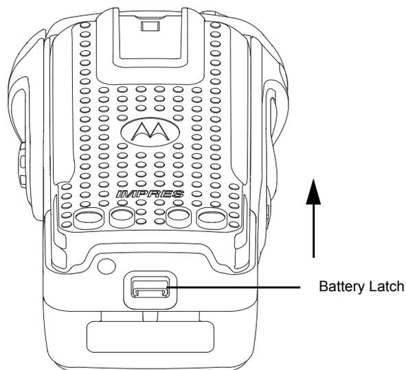
Figure 7-2. Lifting up the battery latch
