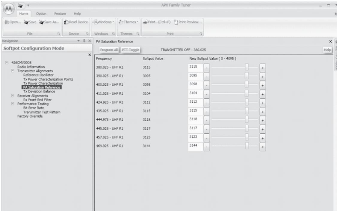
Figure 6-21. PA Saturation Referencing Alignment Screen (UHF1)
