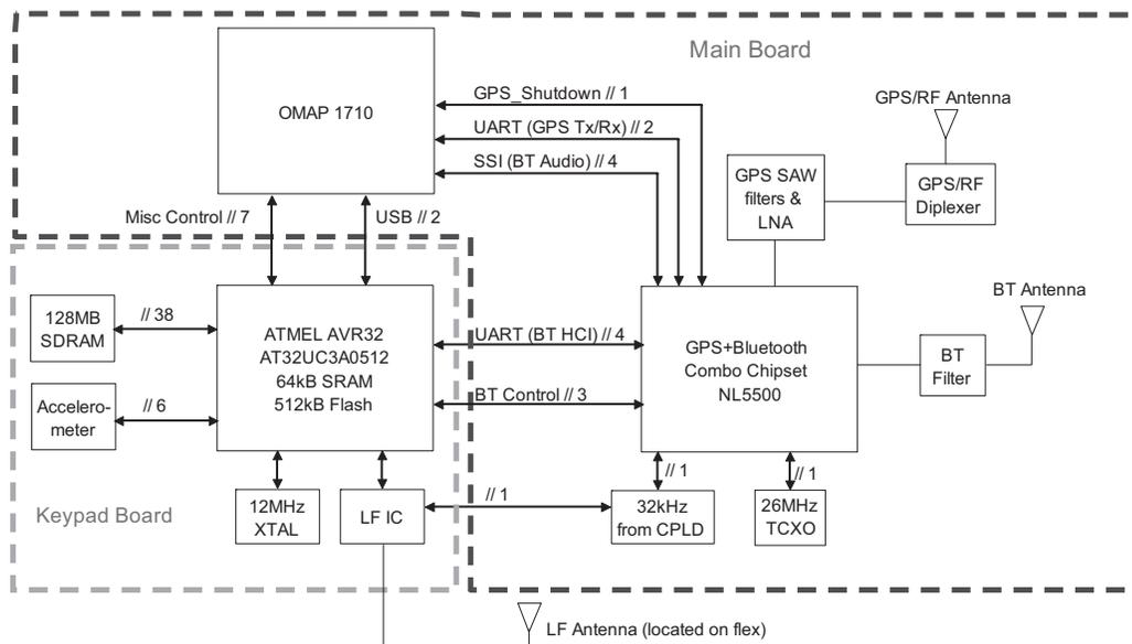
Figure 3-12. GPS/Bluetooth/Accelerometer Block Diagram
