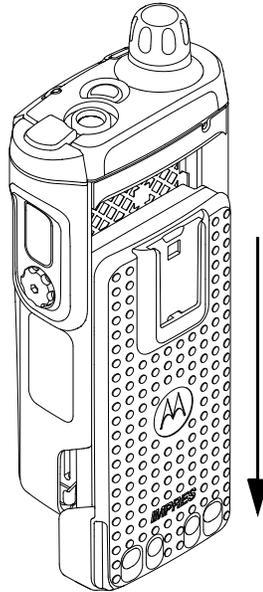
Figure 7-3. Removing the Battery
