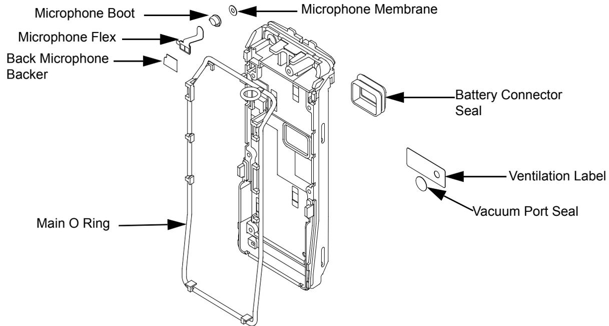
Figure 8-23. Serviceable Components – Chassis Assembly
