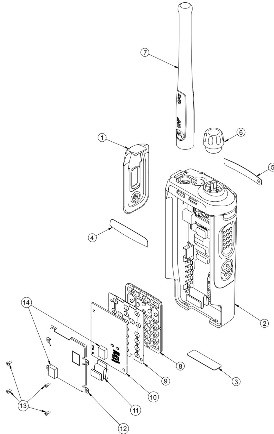
Figure 9-1. APX 1000 Front Kit Exploded View
