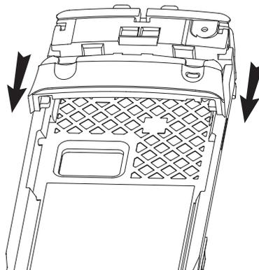
Figure 8-18. Remove the Shroud
