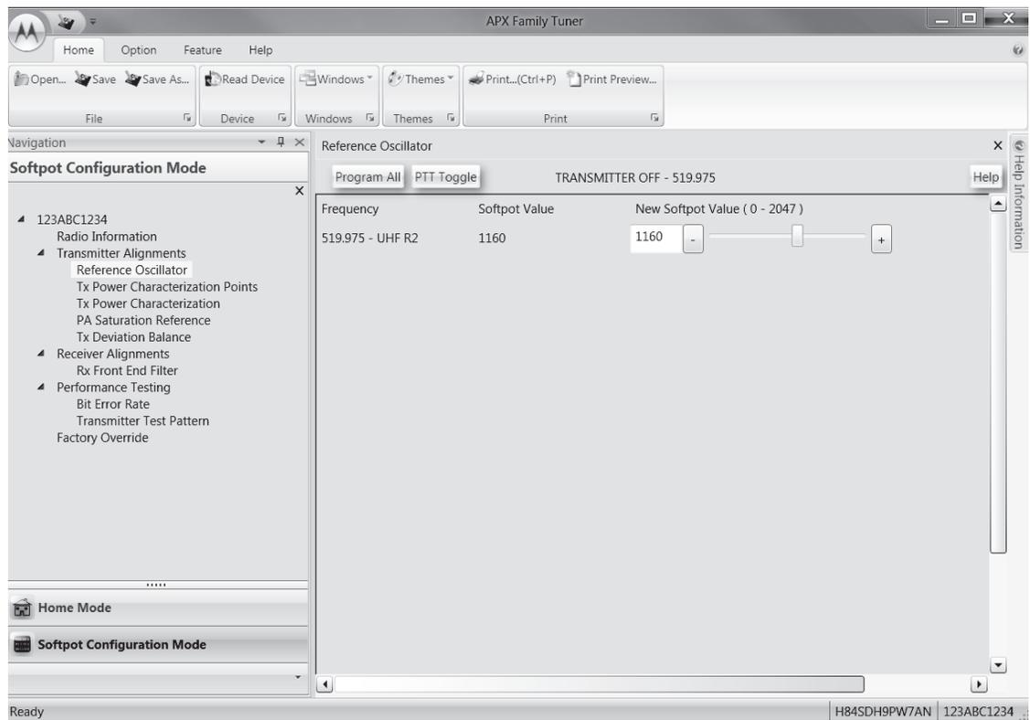
Figure 6-7. Reference Oscillator Alignment Screen (UHF2)
