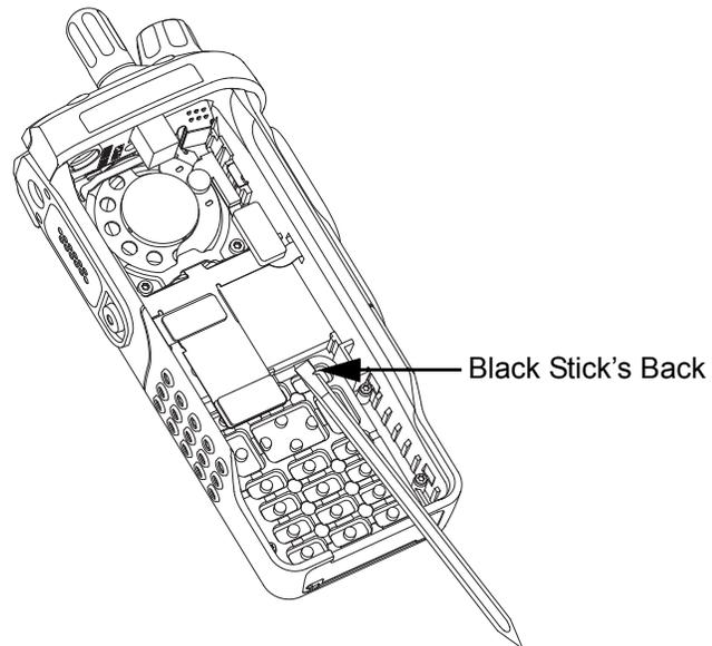
*Figure 8-37. Assemble the Keypad*
