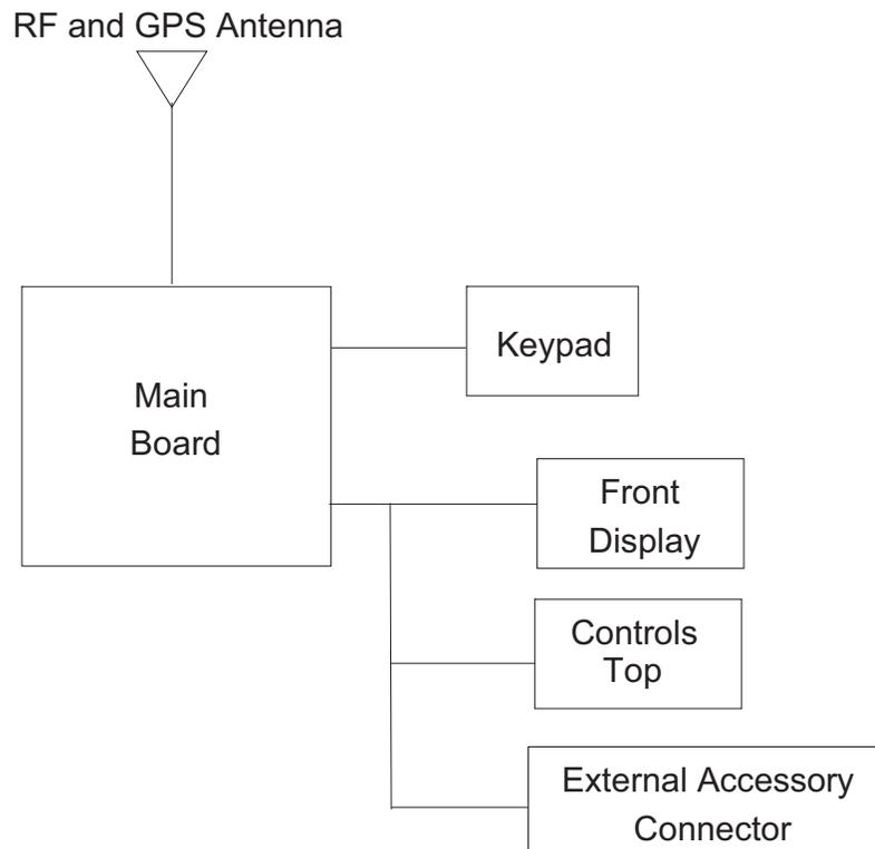
Figure 3-1. APX 1000 Overall Block Diagram
