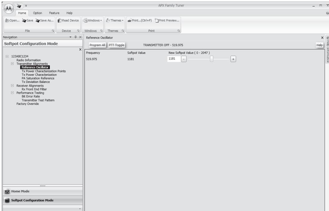
Figure 6-7. Reference Oscillator Alignment Screen (UHF2)
