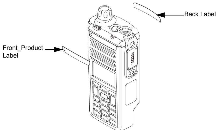
Figure 7-24. Serviceable Components – Main Housing
