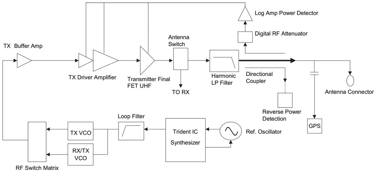
Figure 3-7. Transmitter (UHF1/UHF2) Block Diagram
