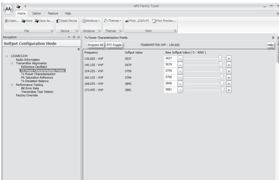
Figure 6-10. Transmit Power Characterization Points Alignment Screen (VHF)
