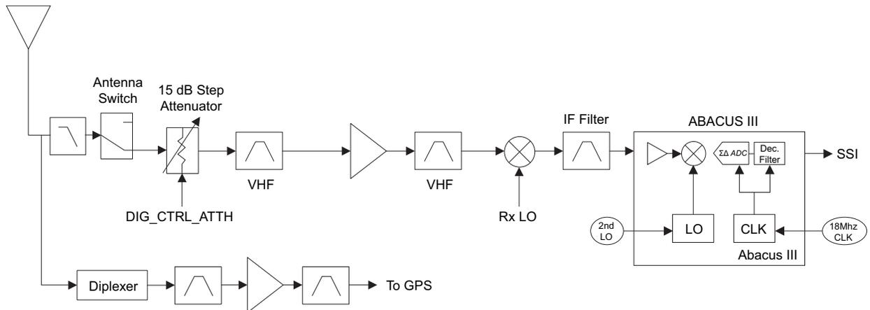
Figure 3-2. Receiver Block Diagram (VHF)
